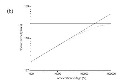
Fig. 2-1. The non-relativistic (solid) and relativistic corrected (dotted) values of (a) the de Broglie wavelength and (b) the velocity for an electron as a function of the applied acceleration voltage. The horizontal line in (b) is the speed of light.
