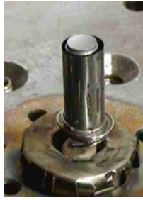
Figure 10. Ba-W Dispenser Cathode
