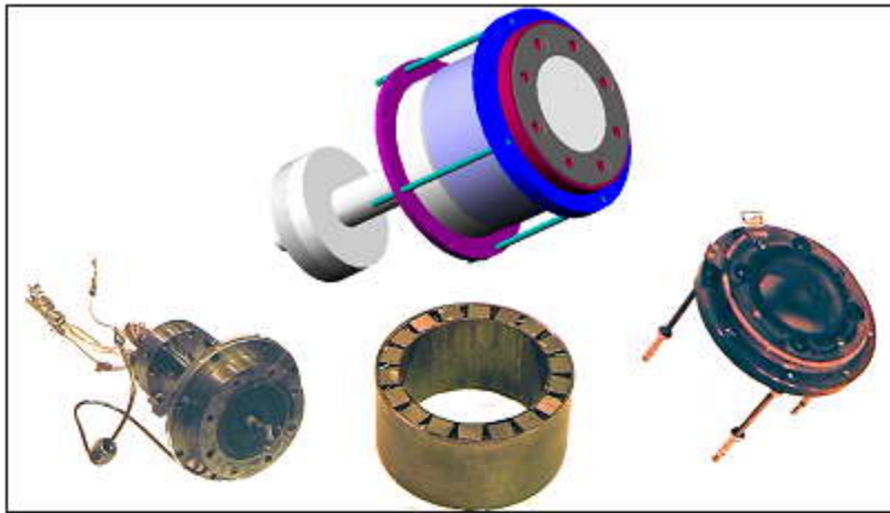
Figure B-1. Thruster Components: Base, Discharge Chamber, and Pole-Piece and Exit Grids
