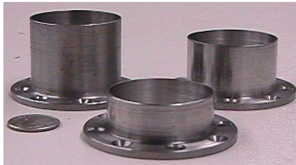
Figure 3.2-1. Micro-Ion Anode of L/D = 1.0, 0.75, and 0.5
