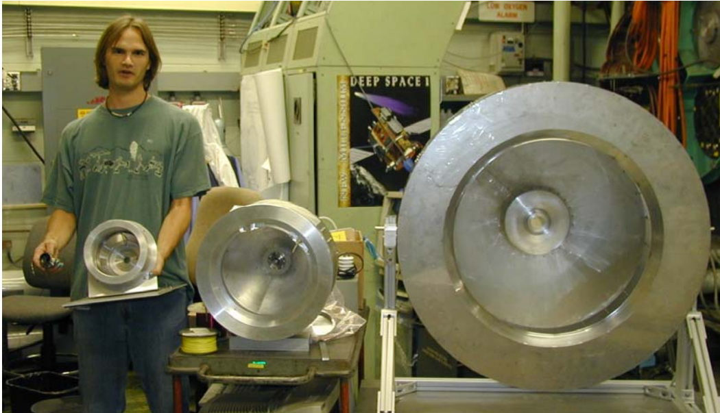
Figure 3.6-3. The Author with (from left to right) the Micro-Ion thruster (3cm), a thruster similar to the 13cm XIPS, NSTAR (30cm), and NEXIS (60cm)
