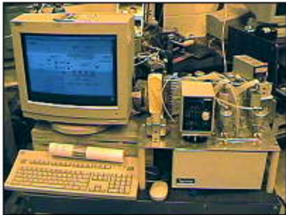
Figure B-6. Propellant Flow Calibration System
