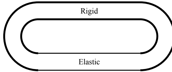
Figure 1.7: Jung's model of the impedance pump
