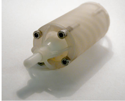
Figure B.1: Photograph of a stereolithography model of the rotary viscous pump.
