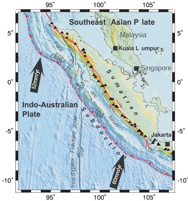
**Figure 1.1** Map of the principal tectonic elements of the Sumatran plate boundary, and on ETOPO2 shaded relief base map. Oblique subduction of the Indian and Australia plates beneath Sumatra is accommodated principally by slip on the Sumatran subduction zone and the dextral Sumatran fault. Volcanoes are triangles. Arrows are plate vectors from GPS.
