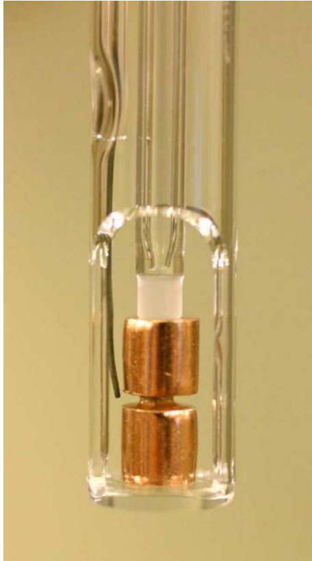
Figure VI-7: Copper-solder-copper stack is loaded into Perkin Elmer TMA7 for accurate control of temperature and load during thermoplastic soldering.
