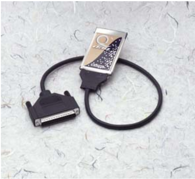
Figure A.8 Quatech IOP-241 : 24 channel digital input / output PCMCIA card
