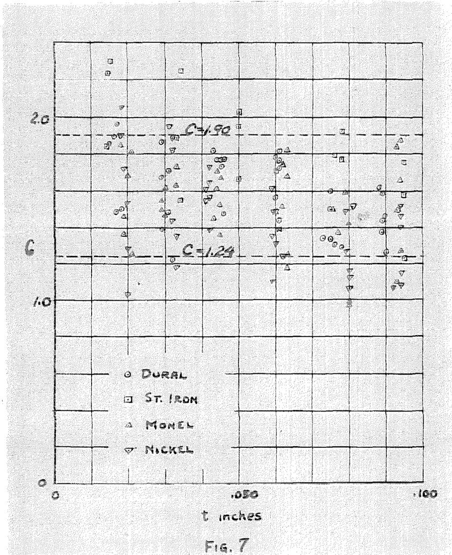
mental values of  $C_F$ , calculated from the experimental loads found in Reference 7 are shown plotted in Fig. 7, and it is seen that nearly all (83%) of the experimental values for  $C_F$  do lie within the range indicated by the above calculations.
