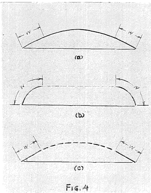
From a purely physical analysis of the problem it seemed reasonable to assume that perhaps most of, or all of the load was carried by that part of the sheet near the edges which was supported and that the center of the sheet was carrying little or no load in the buckled state. In other words, an effective width of the sheet on each side
