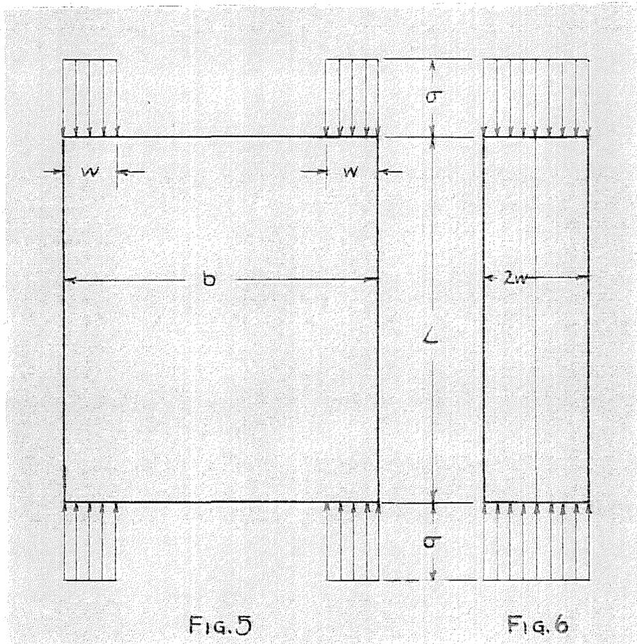
sides of the sheet carried the entire load and that the center of the sheet dropped out of action. See Fig. 5. In order to simplify calculations, there are two possible assumptions that can be made regarding the shape of the sheet in the region "w". The first of these, used by von Karman, assumes that in this region the plate deforms so that the tangents at the end of the two effective widths are parallel. See Fig. 4b. Thus, the center of the sheet can be elimin-
