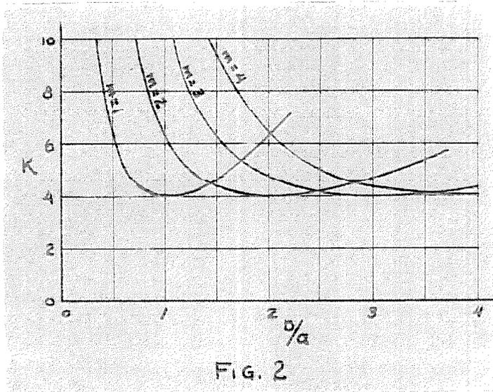
gives the number of half waves in the Y direction, these curves indicate that the buckling tends to give nodal lines forming squares. The wave form in the X direction is one half-wave since  $n = 1$  gave the min-
