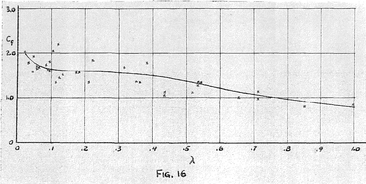
Table I plotted against  $\lambda$ . This plot shows that there is a definite relationship between  $C_f$  and  $\lambda$  even though the curve shown, which is taken as the mean curve through the plotted points, does not agree with any of the theoretical curves in Fig. 15.
