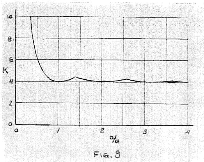
This method of calculating the allowable load for sheet material proved very satisfactory for plates of the thickness used in naval and civil engineering as it was possible to obtain stresses reasonable close to the elastic limit of the material with quite large plates. For example, a sheet of structural steel  $\frac{1}{4}$ " thick could be used up to 30" wide and of any length without having the buckling stress fall below the elastic
