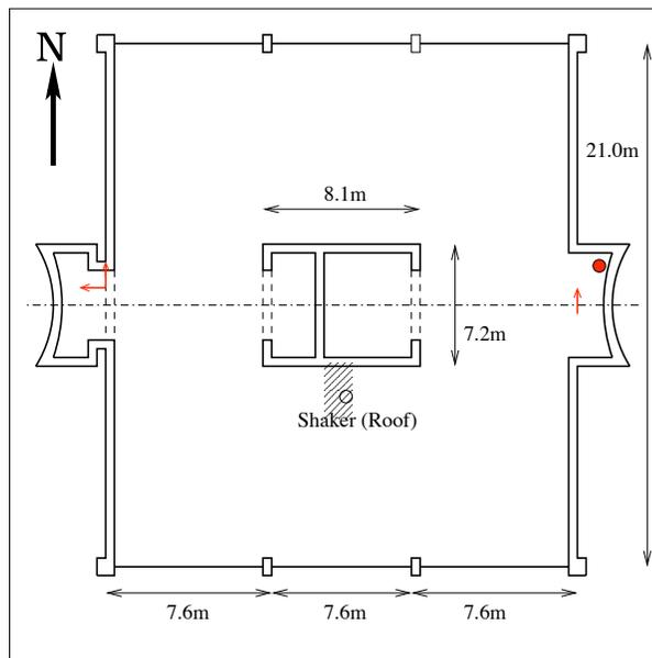
Figure 6.3: Millikan Library — Typical Plan View. The dark circle is the approximate position of CISN Station MIK on the 9<sup>th</sup> Floor, the arrows are the approximate positions and orientations of the 3 USGS channels on each floor (from 1 - Roof).
