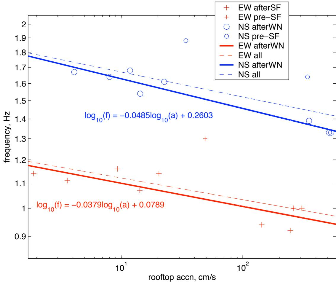
Figure 6.5: Graphical interpretation of Table 1 - Amplitude vs. Frequency, log scaling. For both E-W and N-S, the best fitting least squares solution for all the data is plotted in dashed lines. Outlying data from tests and earthquakes prior to main permanent natural frequency shift (pre- Whittier Narrows for N-S; pre- San Fernando for E-W) are removed from dataset for the solid line regressions, with labelled functional form.
