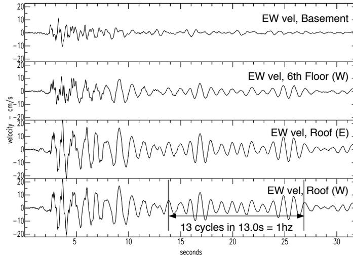
Figure 6.6: East-West components of CR-1 array in Millikan Library, recorded during the M6.1 Whittier Narrows earthquake  $\Delta = 19km$  - velocity timeseries. The top trace is from the basement, the second is from the 6<sup>th</sup> floor, and the last two are from the roof. The last trace includes a sample of how the fundamental frequency of the building is estimated, after the main energy (seen from the basement trace) has passed.
