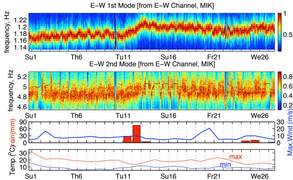
Figure 6.20: Spectrogram of Fundamental and 2<sup>nd</sup> mode frequencies for E-W mode during February 2003, a time of heavy rainfall. 1 hour spectrogram windows, scaled by the maximum value, linear colourbar. JPL weather on bottom. Note correlation between rises in both natural frequencies and heavy rainfall.
