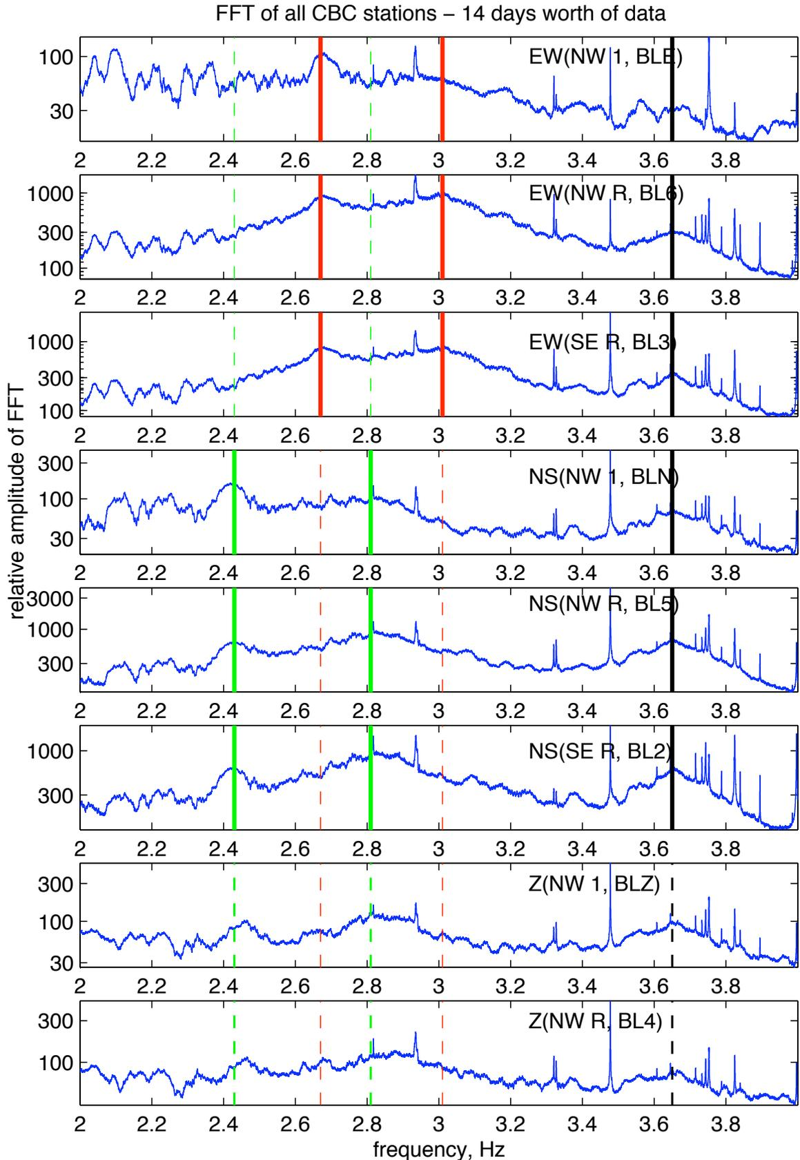
Figure 6.10: Broad Center — Stacked FFT data from 14 days in February. Suspected natural frequencies shown by vertical bars: red - EW (2.67, 3.01 Hz); green - NS (2.43, 2.81 Hz), black - torsional (3.65 Hz).
