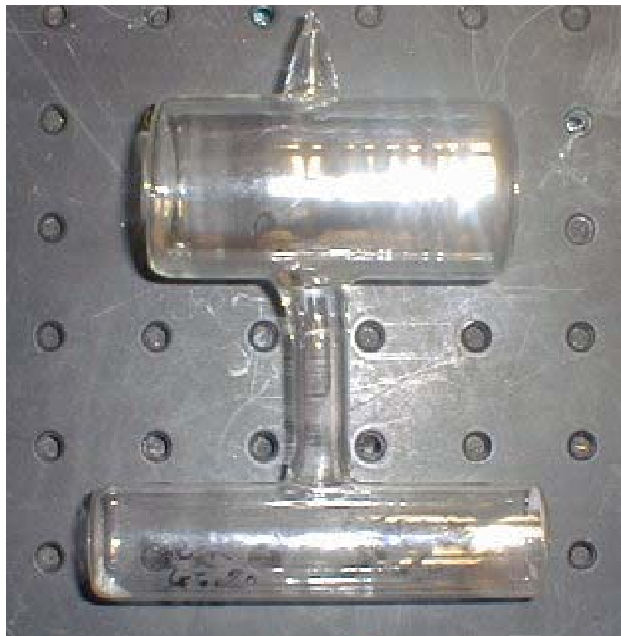
Figure 3.1: A double-chamber cell used in the experiments. The background is an optical table with threaded holes with one inch spacing.
