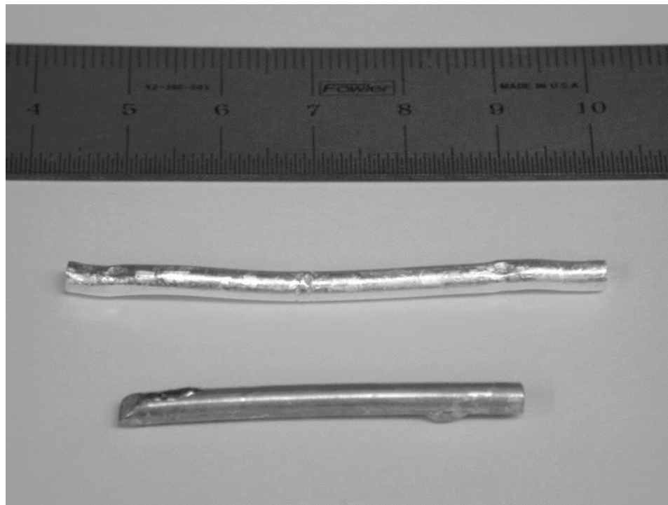
Figure D.1: Typical 5N silver before and after annealing. Note the millimeter-sized grains on the annealed sample (top).
