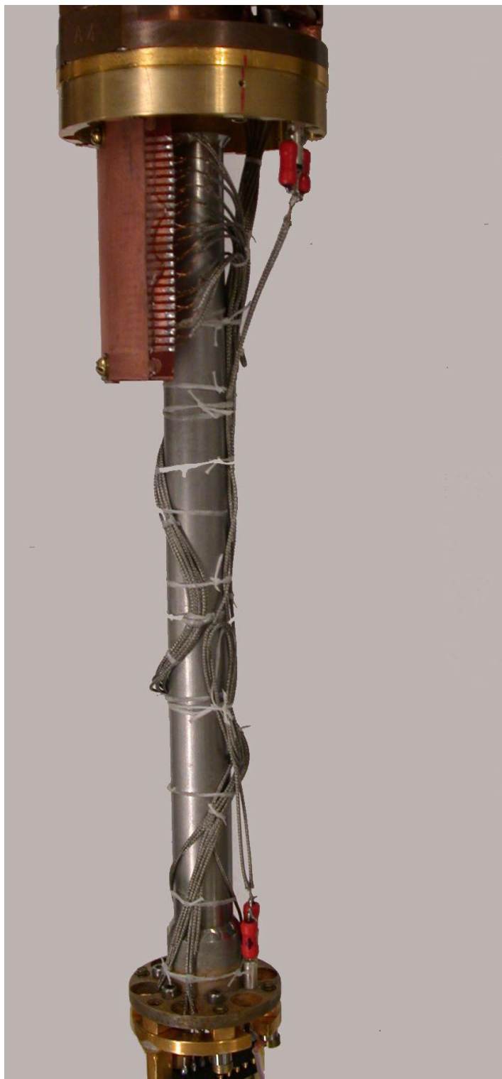
Figure C.5: Photo of KelvinOx 25 tail piece, with sample mount attached on the bottom.
