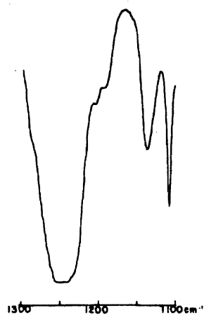
Fig. 5 Part of the infrared spectrum of a carbon tetrachloride solution of the acetolysis products of 2-ferrocenylpropyl p-toluenesulfonate
