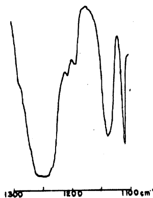
Fig. 10 Part of the infrared spectrum of a carbon tetrachloride solution of 1-ferrocenyl-2-propyl acetate
