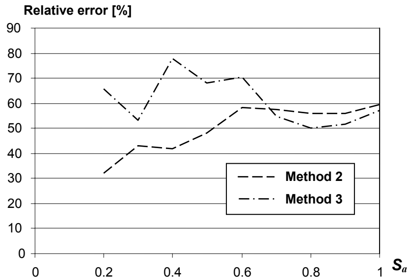
Figure 4.18. Relative errors of estimation of E[N_i] by different methods as a function of spectral acceleration for the axial force-flexure interaction model, ground motion LA15.
