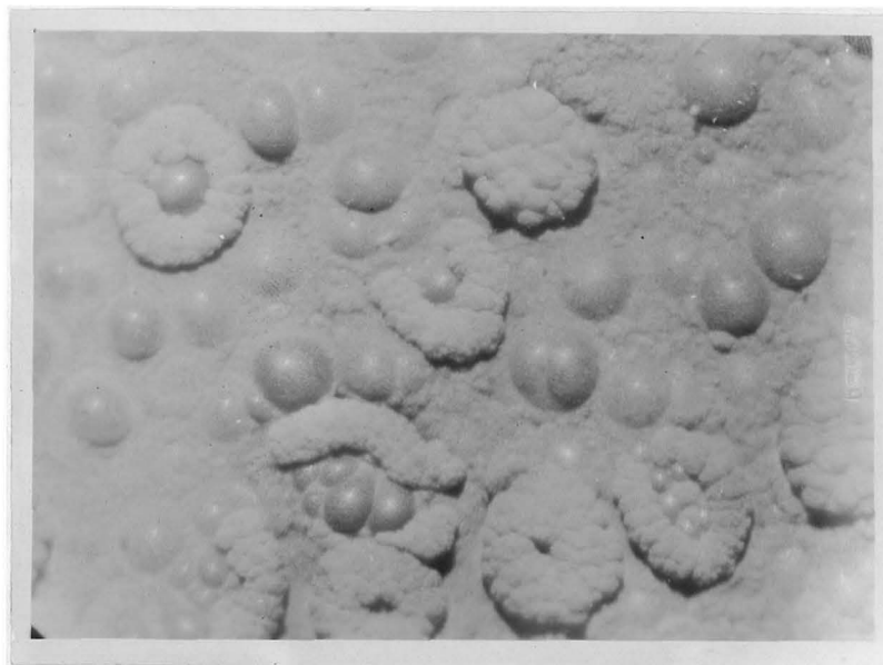
Fig. 16. Crystalline growth above the fusion of Fig. 3. The grapelike clusters are believed to be cristobalite, the smooth domes glass. (X75)
