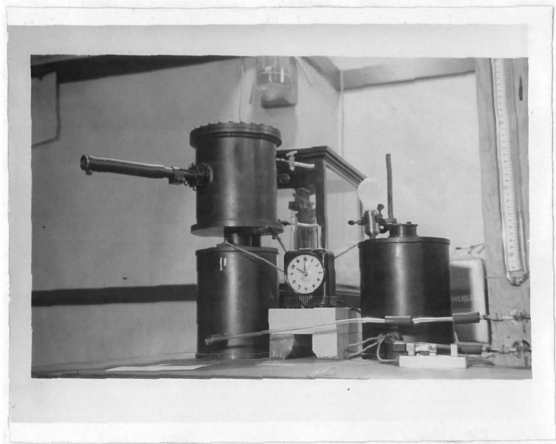
Fig. 22b. Removable head, bifilar electrometer with two ionization chambers.
