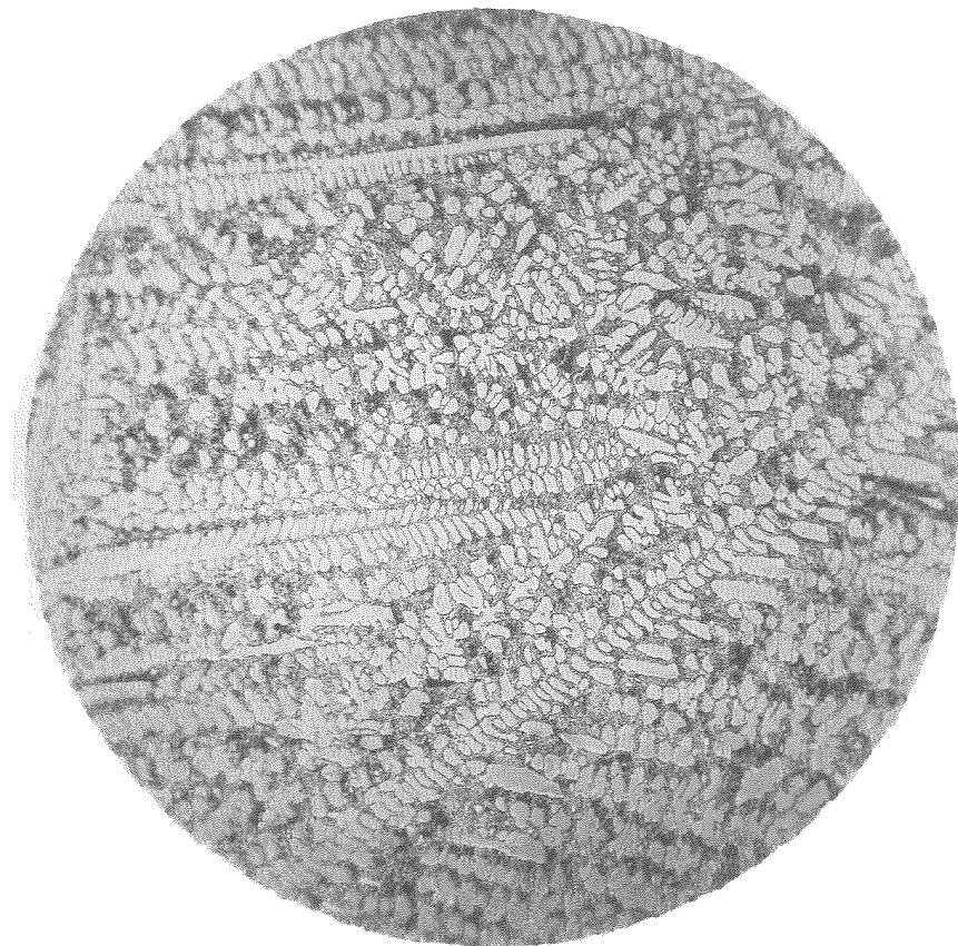
Fig. 141 (225B) As cast Magnification 100X Etch Murakami
