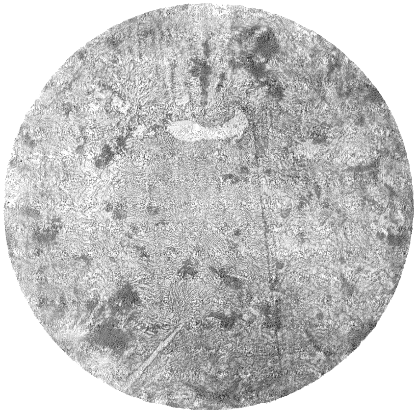
Fig. 109 (292B-3) As cast Magnification 1000X Etch 5% Picrol
