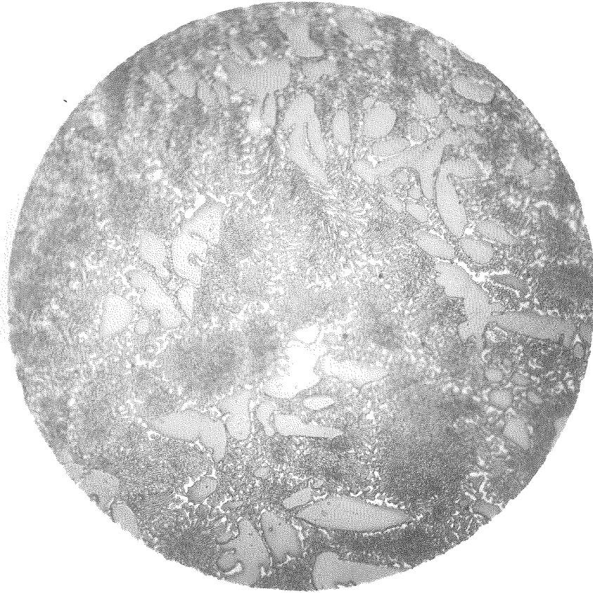
Fig. 69 (13-2) As cast Magnification 500X Etch Murakami
