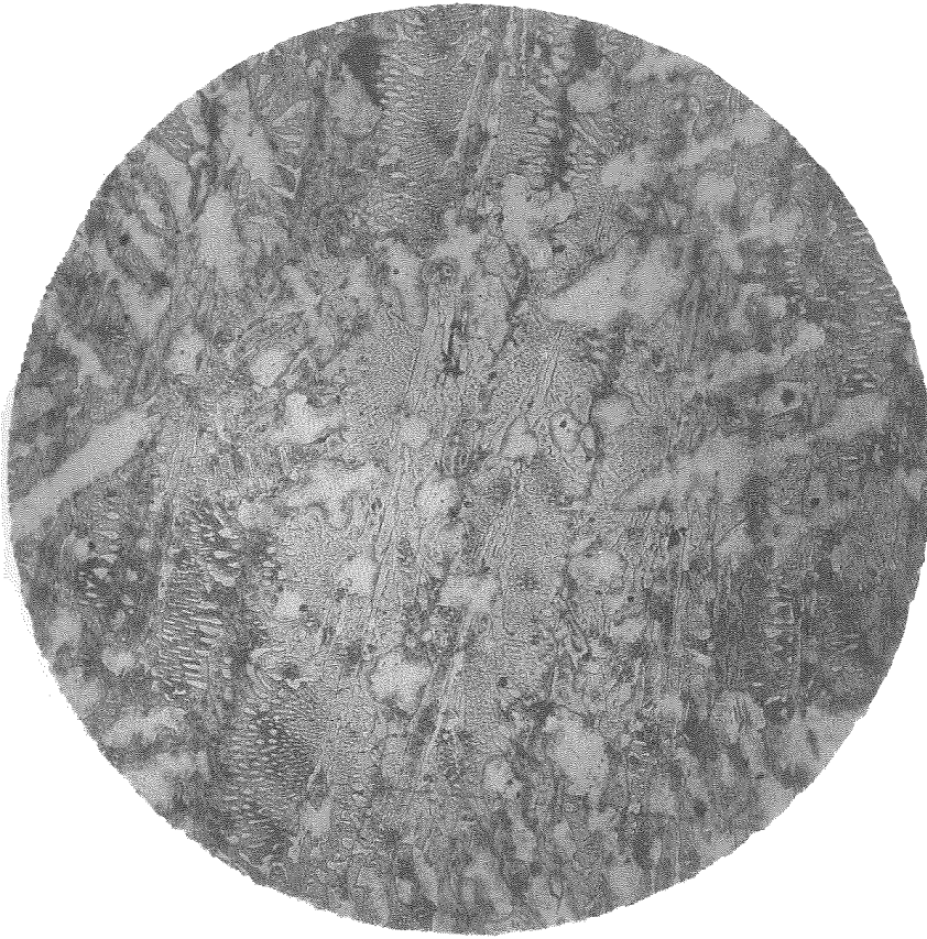
Fig. 118 (270BA) As cast Magnification 100X Etch Murakami
