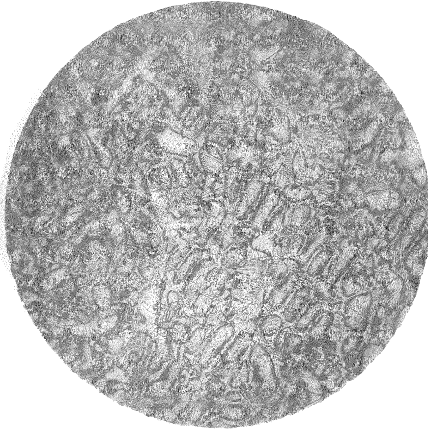
Fig. 124 (400B1) As cast Magnification 100X Etch Murakami
