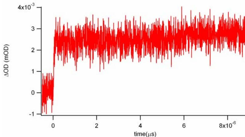
**Figure 4.8.** Transient absorption of Re126/W122/Az( $\text{Cu}^+$ ) with quencher. 10  $\mu\text{M}$  Ru124/W122/Az( $\text{Cu}^+$ ), 10 mM  $\text{Ru}(\text{NH}_3)_6\text{Cl}_3$ , 25 mM  $\text{KP}_i$ , pH 7.28.  $\lambda_{\text{ex}} = 355$  nm,  $\lambda_{\text{obs}} = 628$  nm
