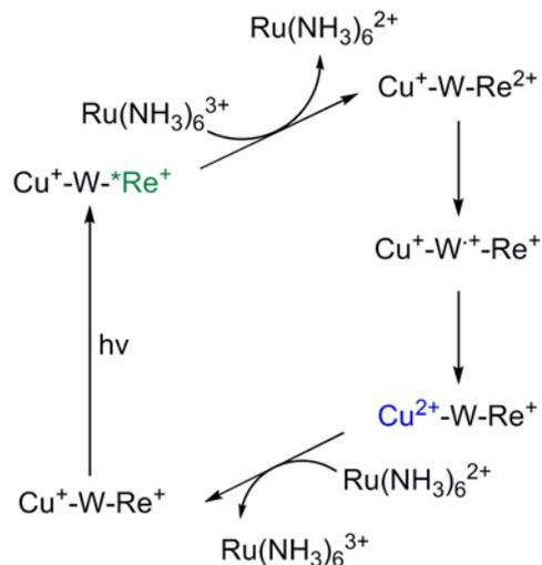
**Scheme 4.3.** Events after sample excitation in Re126/W122/Az(Cu<sup>+</sup>) with Ru(NH<sub>3</sub>)<sub>3</sub><sup>3+</sup>. Colors indicate species observed spectroscopically.
