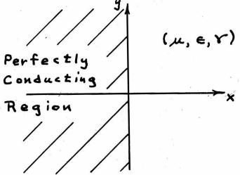
The tangential components of E must vanish on the boundary, by the definition of a perfect conductor. So we have
