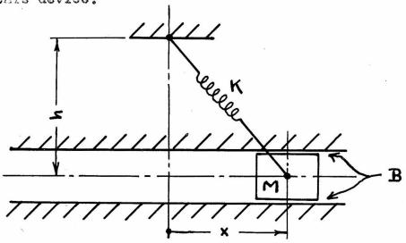
It has only one degree of freedom. It is composed of a rigid mass M and a linear (Booke's-Law) spring of stiffness parameter K, whose unstretched length is h. Viscous friction (retarding force proportional to relative velocity) affects the mass, with coefficient B. Its equation of motion is (by Newton's Second Law):
