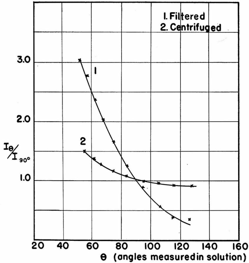
Figure 14. The angular scattering of a nitrocellulose solution after filtration and after centrifugation. (Figure is from an article by Blaker, R. H., Badger, R. M., and Gilman, T. S., *J. Phys. and Coll. Chem.*, 53, 794 (1949).)
