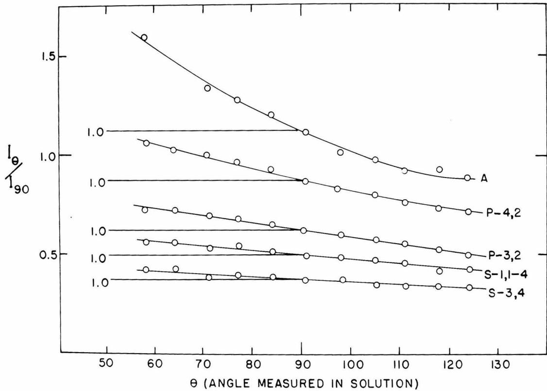
Figure 22. The angular distribution of scattering for five nitrocellulose fractions
