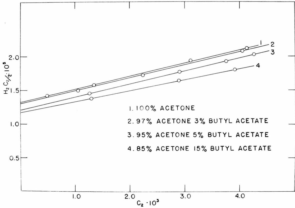
Figure 30. Turbidity of nitrocellulose in acetone-butyl acetate mixtures
