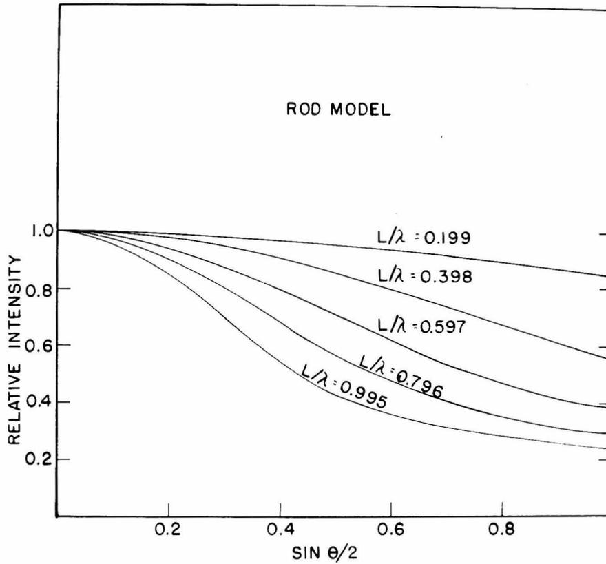
Figure 16. Relative intensity of scattering as a function of angle for the rod model
