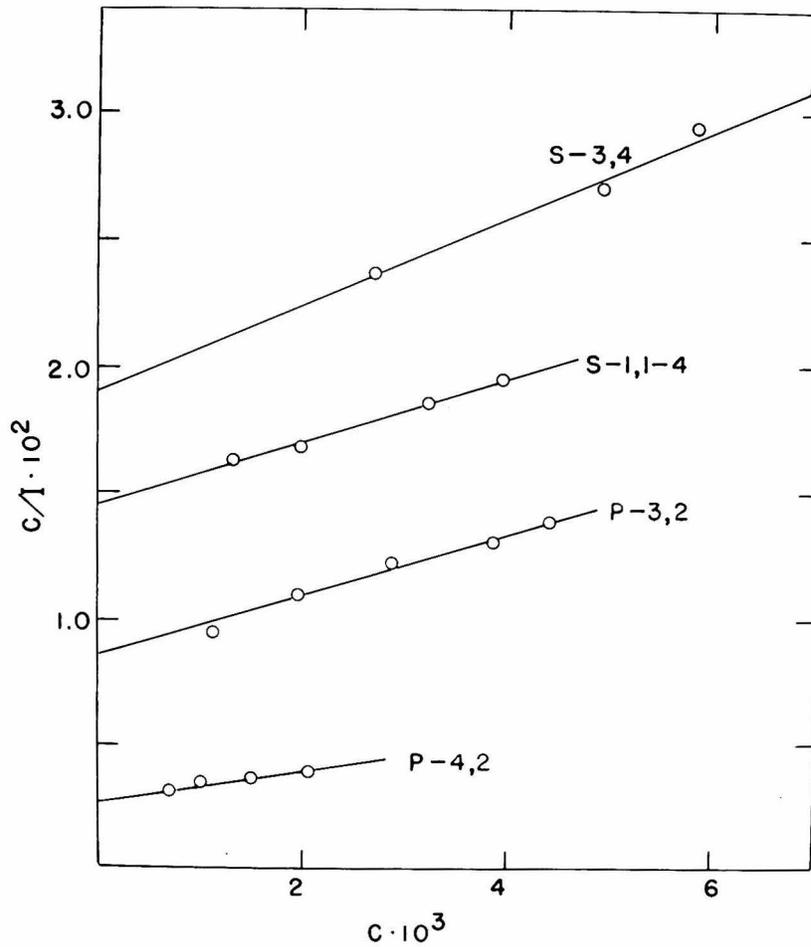
Figure 21. A plot of  $c/I$  versus  $c$  for four nitrocellulose fractions.  $c$  is concentration expressed as weight fraction.  $I$  is the ratio of the  $90^\circ$  scattering of the solution to that of carbon disulfide.
