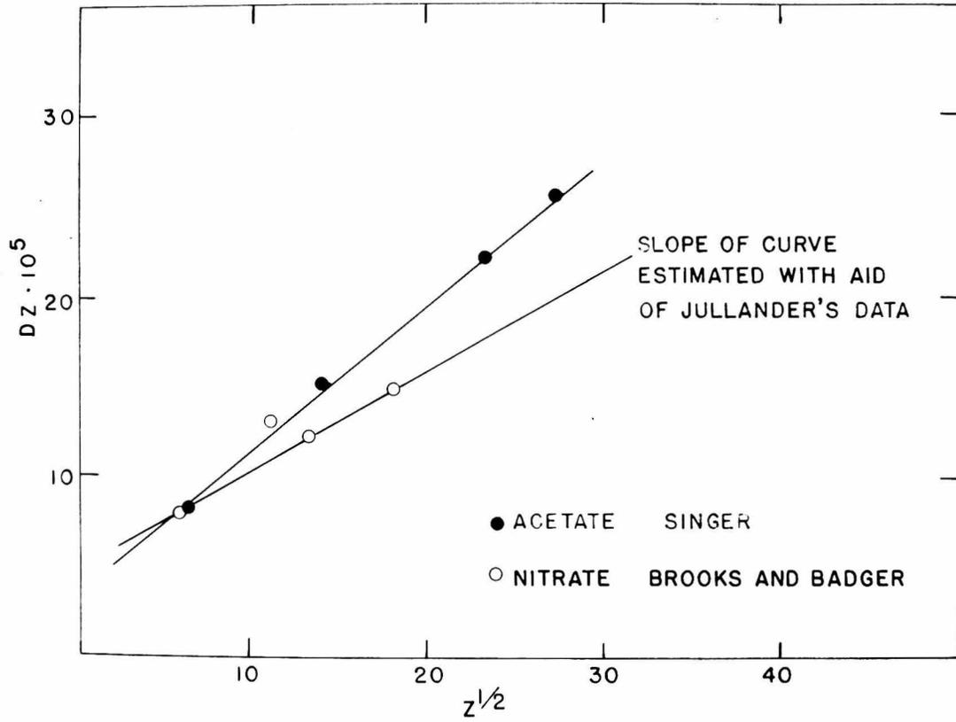
Figure 26. Variation of  $DZ$  with  $z^{1/2}$  for nitrocellulose and cellulose acetate
