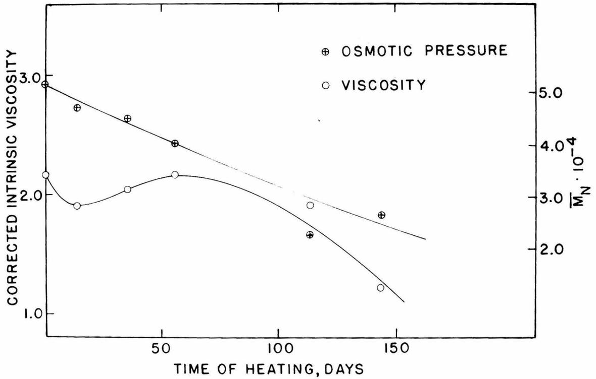
Figure 6. Viscosity and osmotic pressure data for nitrocellulose from heated powders
