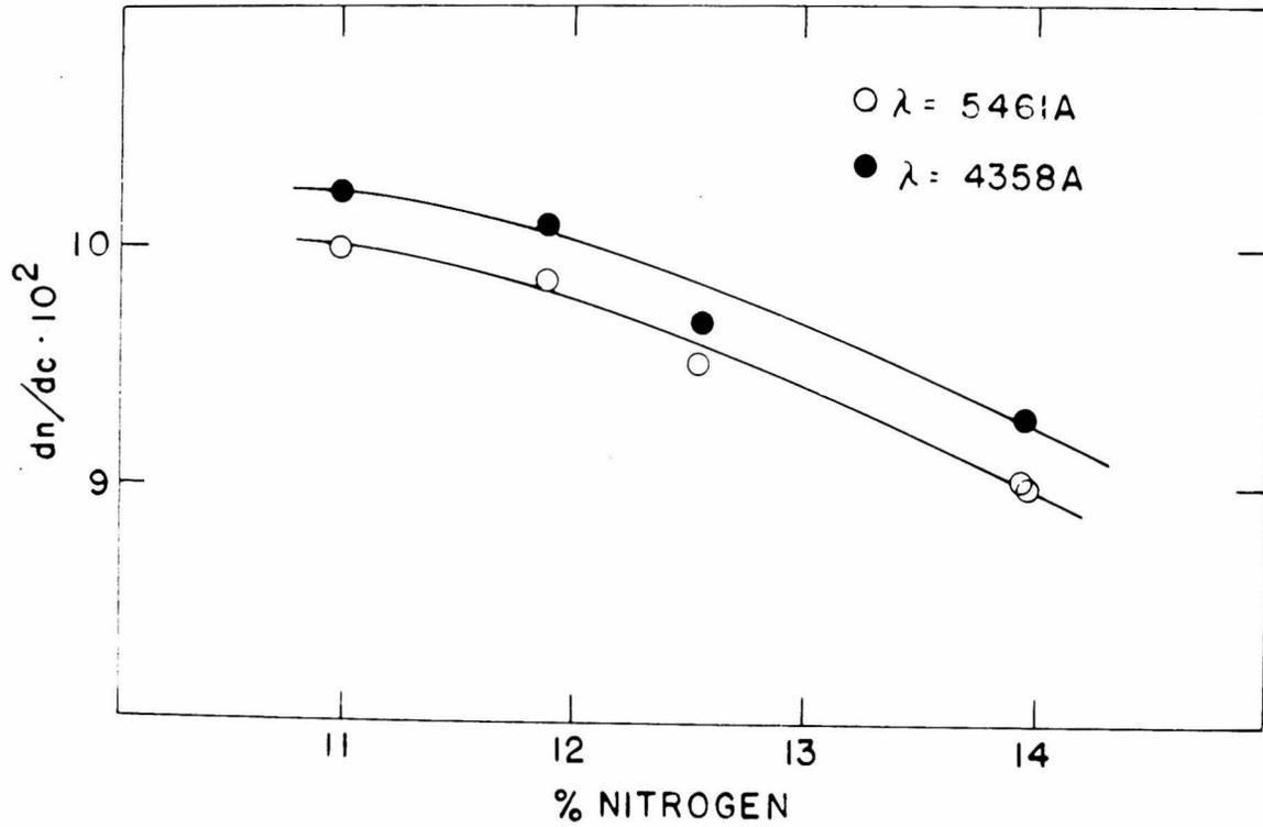
Figure 20. Variation of refractive index increment of nitrocellulose with nitrogen content
