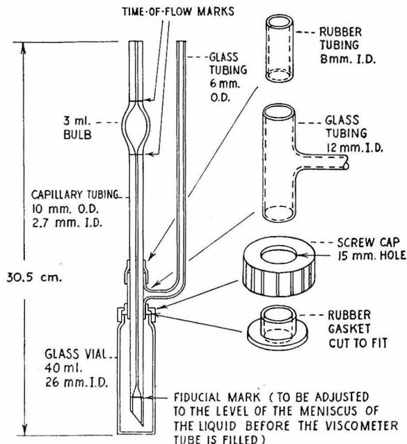
Figure 1. Diagram of Viscometer
