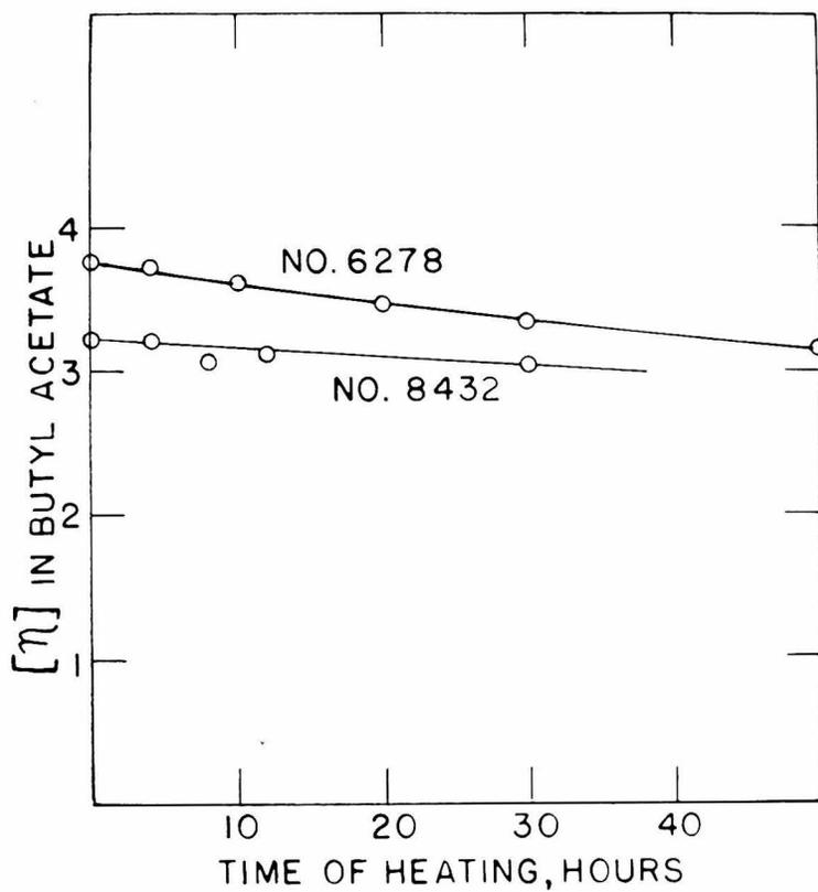
Figure 1. Change of intrinsic viscosity with time of heating at  $100^{\circ}$  C. Nitrocellulose No. 6278 contains 13.4 per cent nitrogen. Nitrocellulose No. 8432 contains 12.6 per cent nitrogen.
