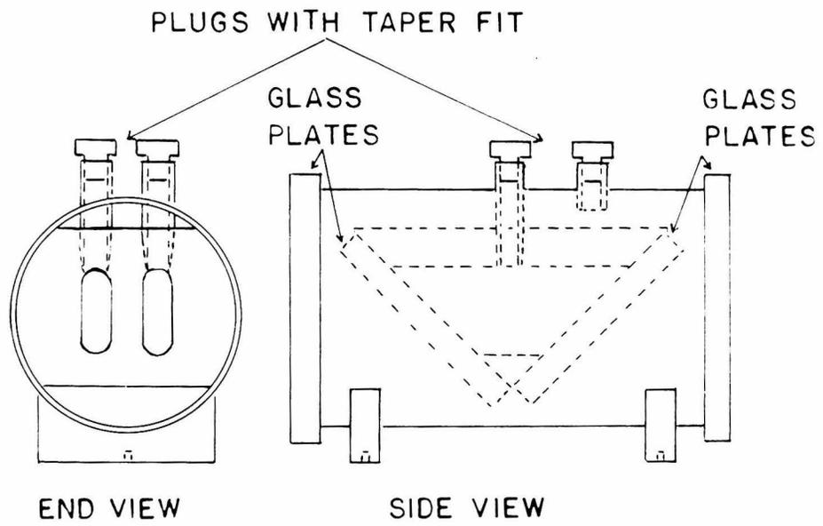
Figure 9. Prism of differential refractometer
