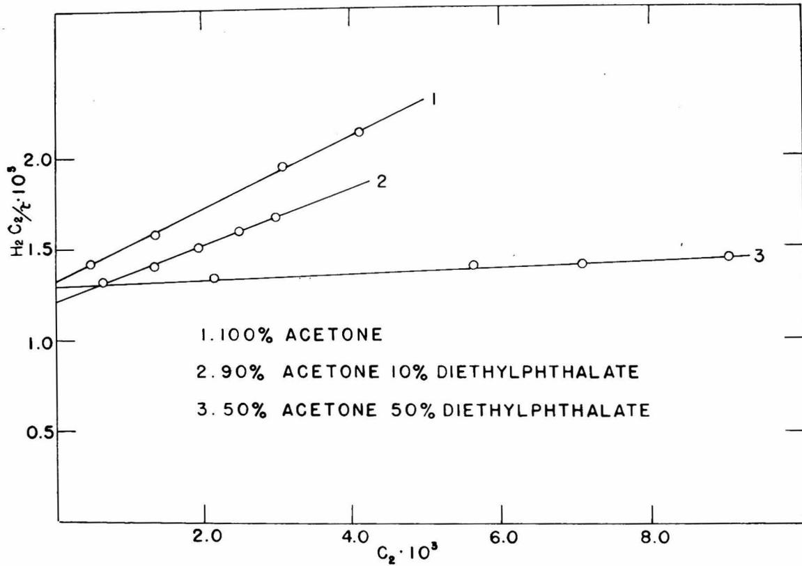
Figure 32. Turbidity of nitrocellulose in acetone-diethyl phthalate mixtures
