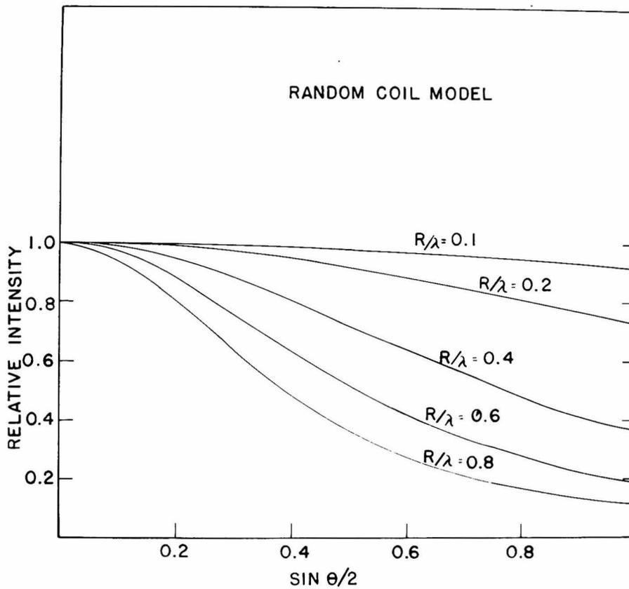
Figure 17. Relative intensity of scattering as a function of angle for the random coil model
