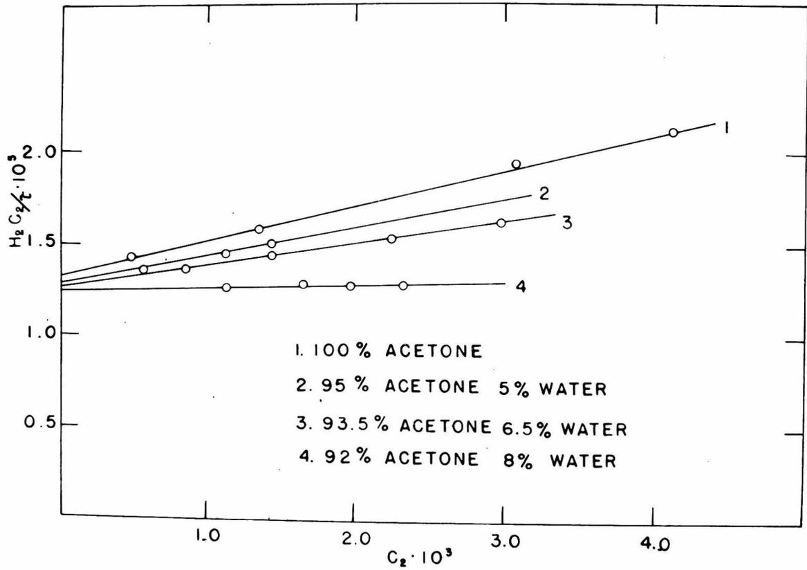
Figure 28. Turbidity data for nitrocellulose in acetone-water mixtures
