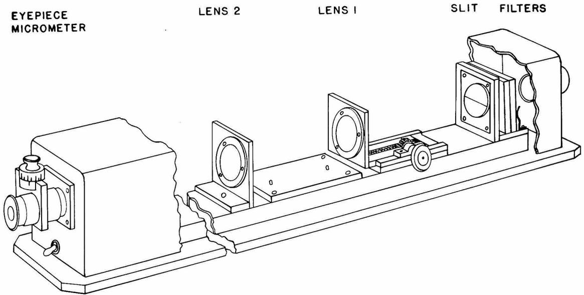
Figure 8. Differential refractometer
