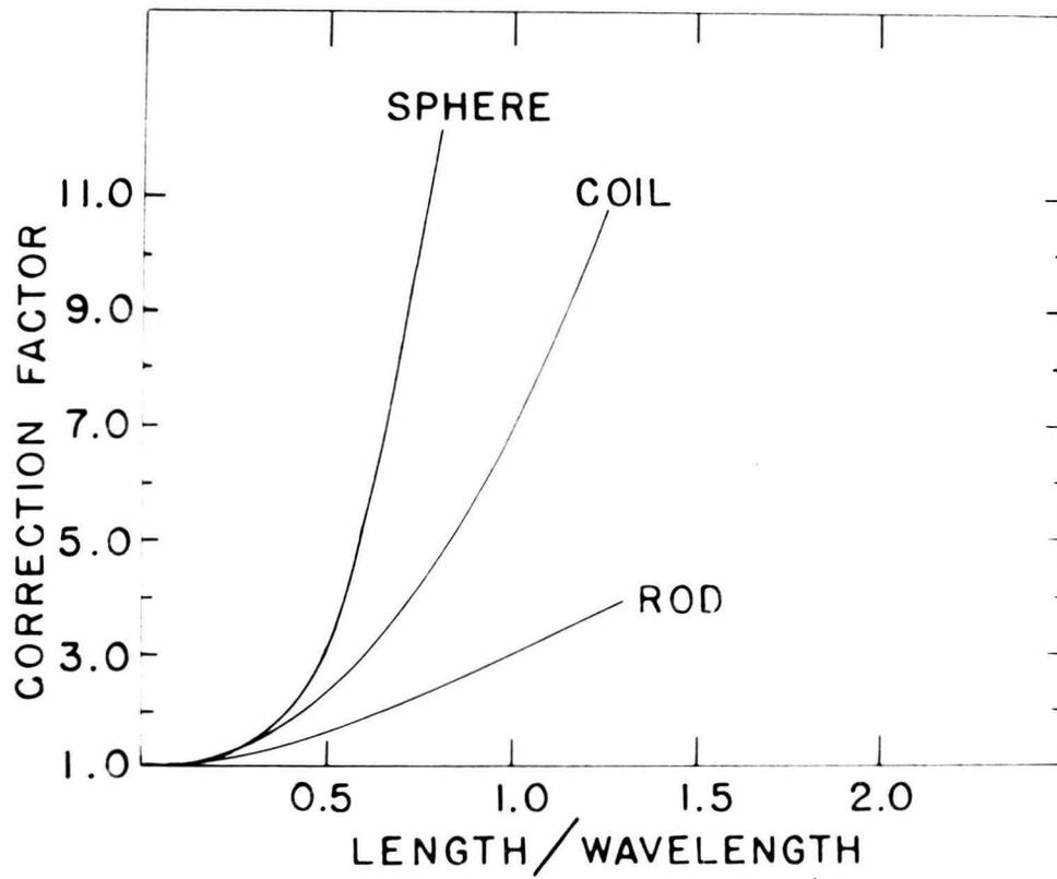
Figure 19. Correction factor as a function of the ratio of the characteristic dimension to wave length of light for three models
