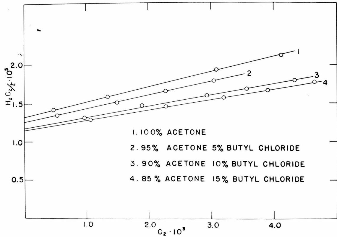
Figure 31. Turbidity of nitrocellulose in acetone-butyl chloride mixtures
