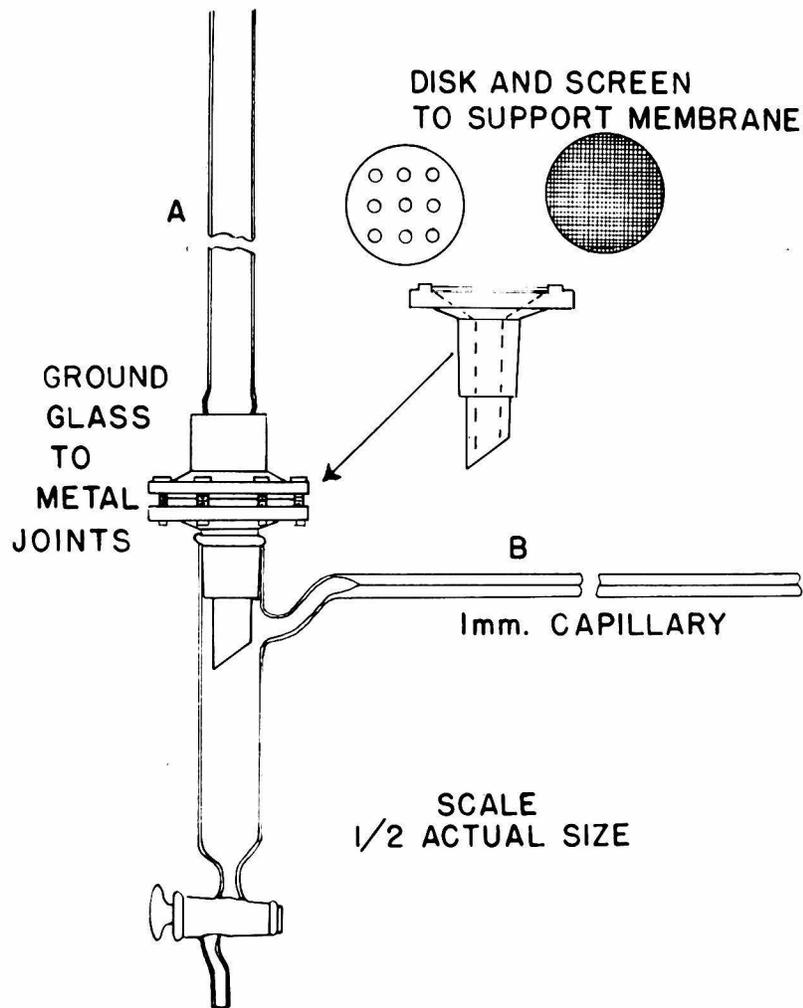
Figure 2. Apparatus to measure permeability of membranes
