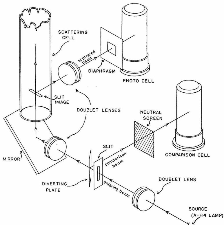
Figure 10. Scheme of the optical path in the photoelectric photometer. (Figure is from an article by Blaker, R. H., Badger, R. M., and Gilman, T. S., J. Phys. and Coll. Chem., 53, 794 (1949).)
