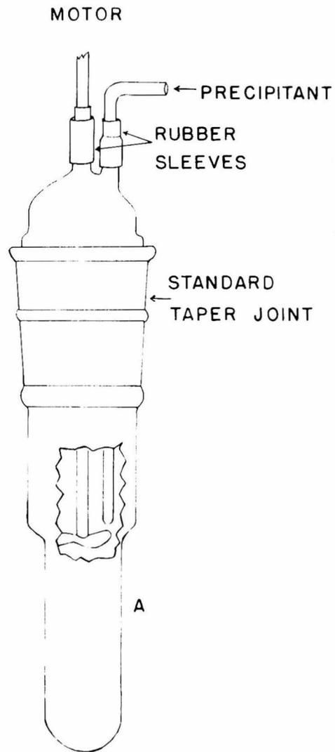
Figure 7. Precipitation cell
