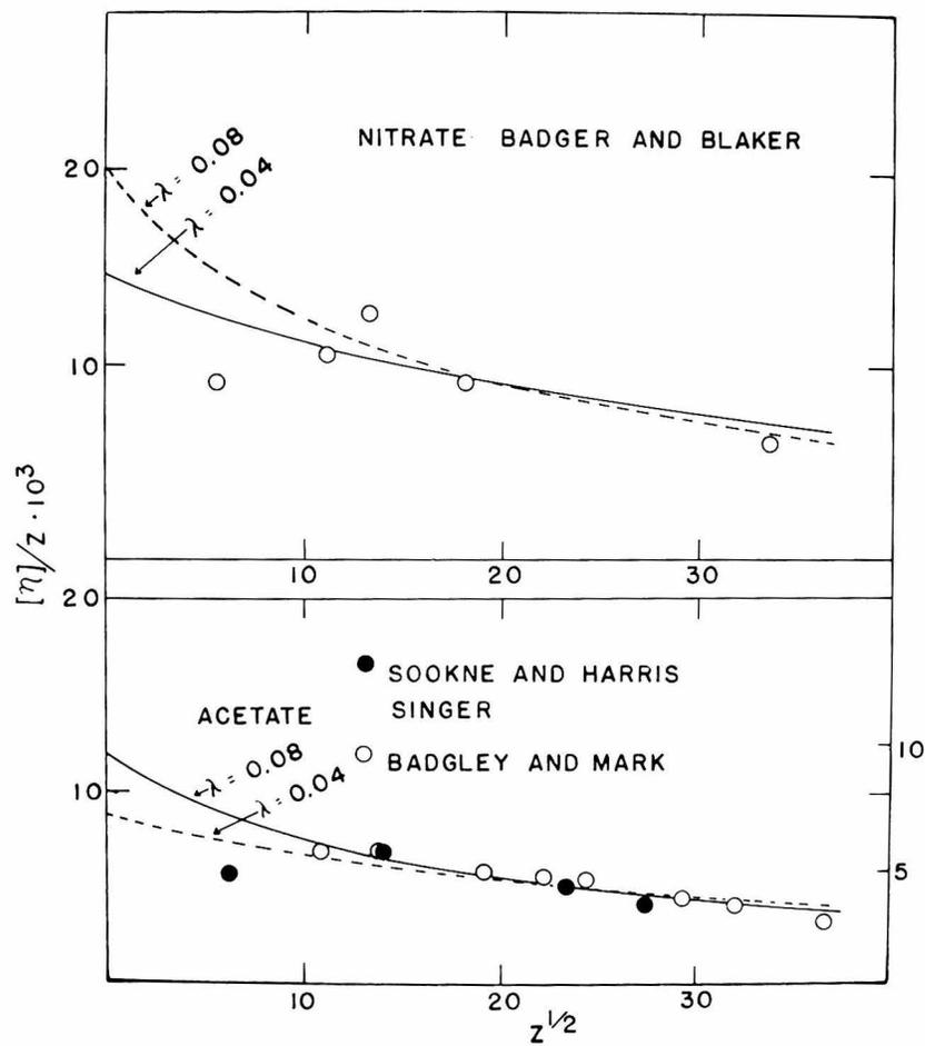
Figure 27. A comparison of experimental values of  $[\eta]/z$  with those predicted by the K-R theory. The scale of the right ordinate is for the data of Badgley and Mark.
