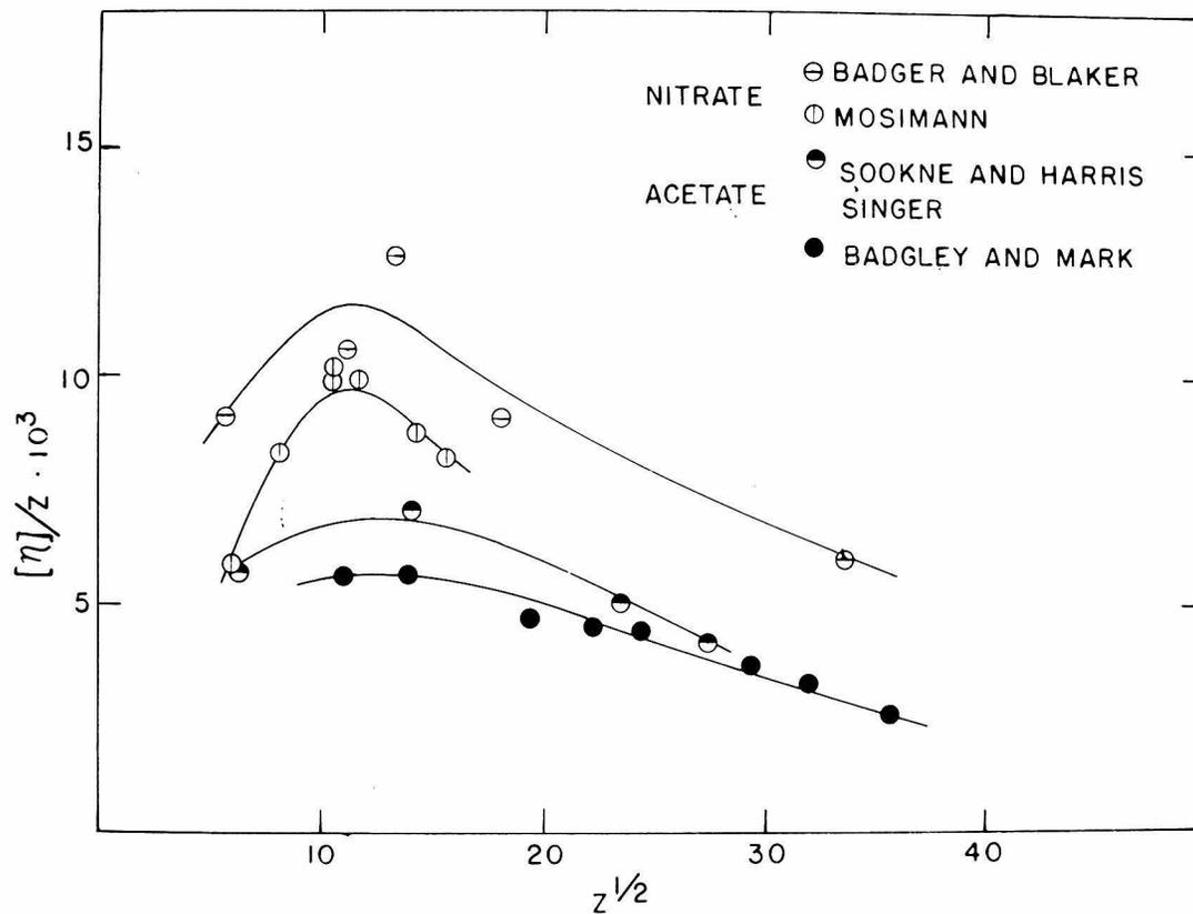
Figure 25. Variation of  $[\eta]/z$  with  $z^{1/2}$  for nitrocellulose and cellulose acetate
