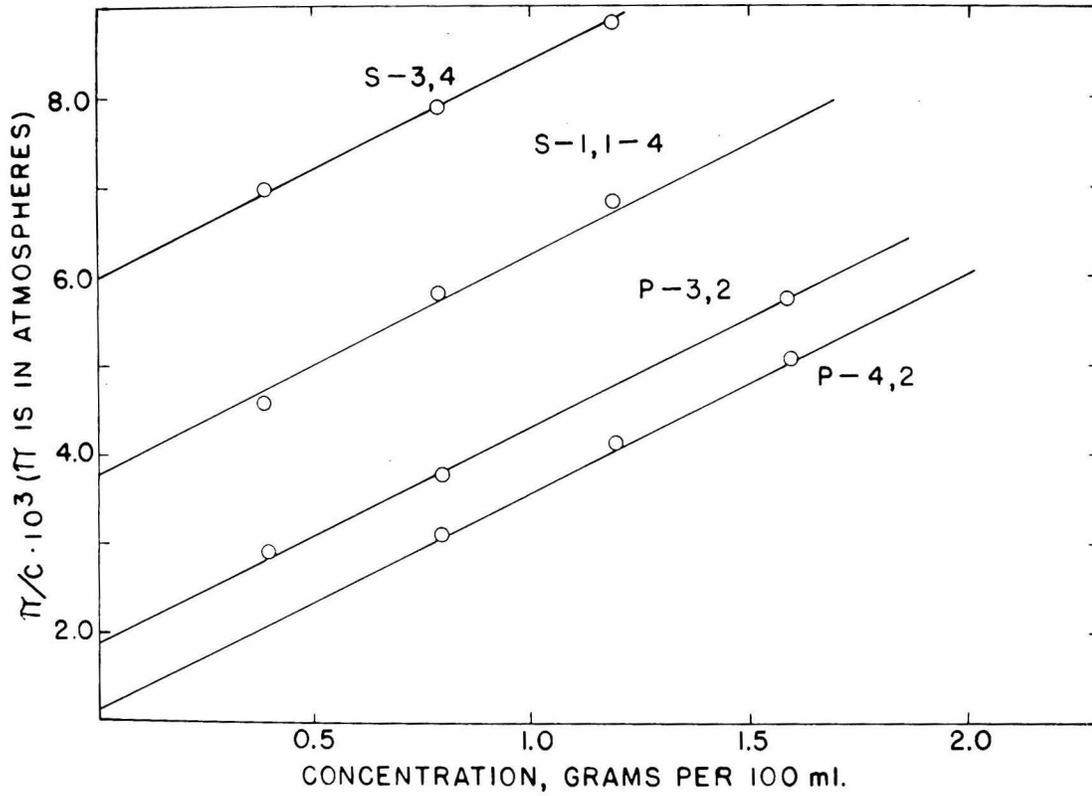
Figure 5. Osmotic pressure data for four nitrocellulose fractions in acetone solution
