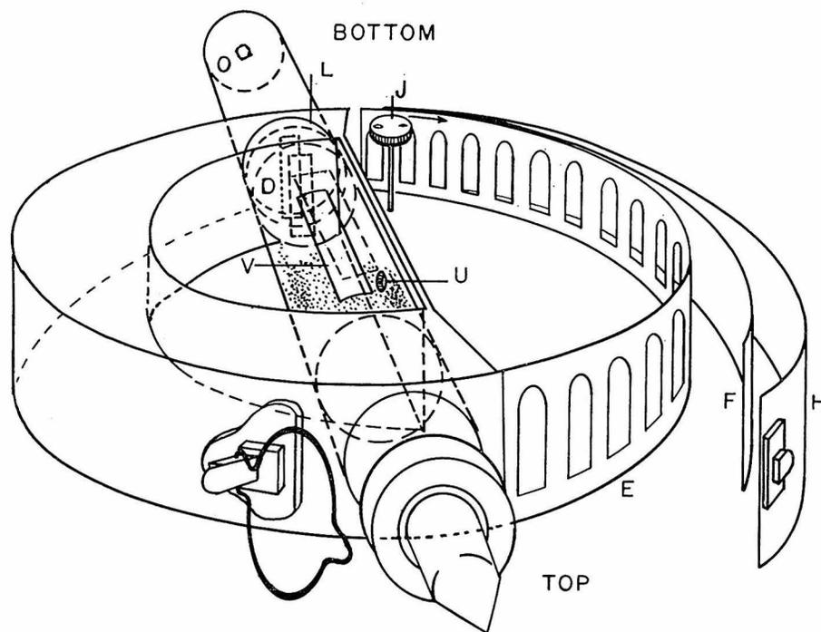
Figure 12. Camera for the determination of the angular distribution of scattering. (Figure is from an article by Blaker, R. H., Badger, R. M., and Gilman, T. S., *J. Phys. and Coll. Chem.*, 53, 794 (1949).)
