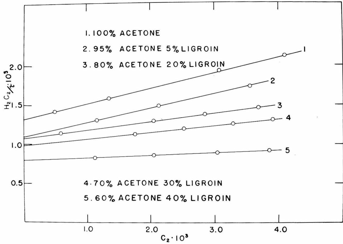
Figure 29. Turbidity of nitrocellulose in acetone-ligroin mixtures
