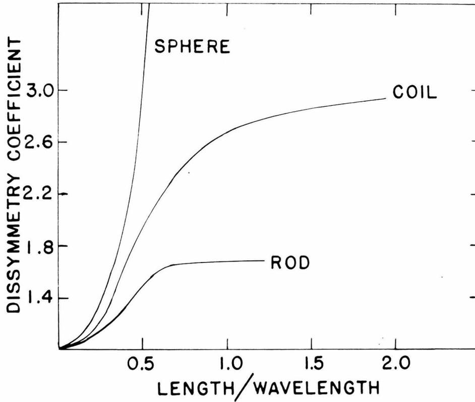
Figure 18. Dissymmetry coefficient as a function of the ratio of the characteristic dimension to wave length of light for three models
