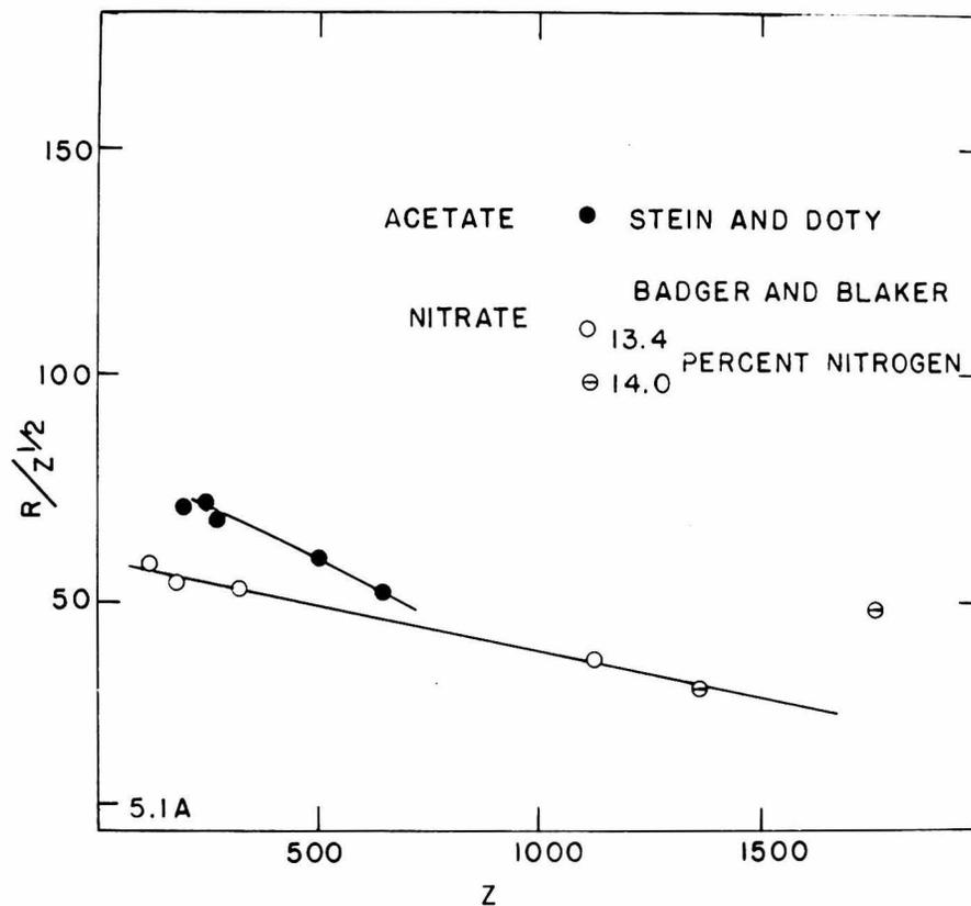
Figure 24. Variation of  $R/Z^{1/2}$  with Z for nitrocellulose and cellulose acetate
