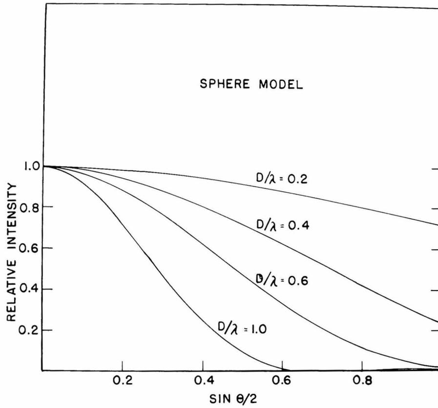
Figure 15. Relative intensity of scattering as a function of angle for the sphere model
