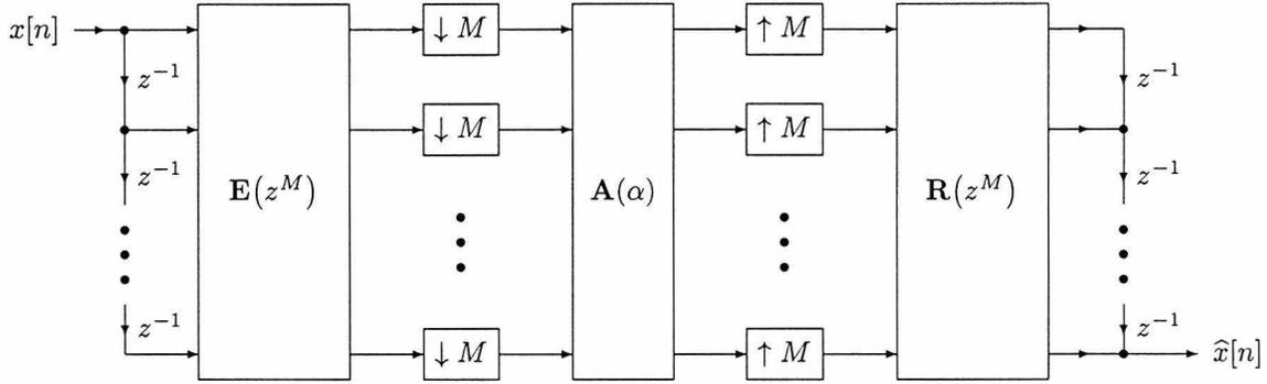
Figure 3.5: Polyphase form of the  $M$ -channel maximally decimated filter bank implemented with the FDFT
