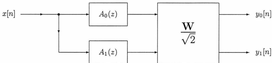
Figure 3.1: Implementation of two transfer functions using the sum and difference of two allpass filters (DFT)
