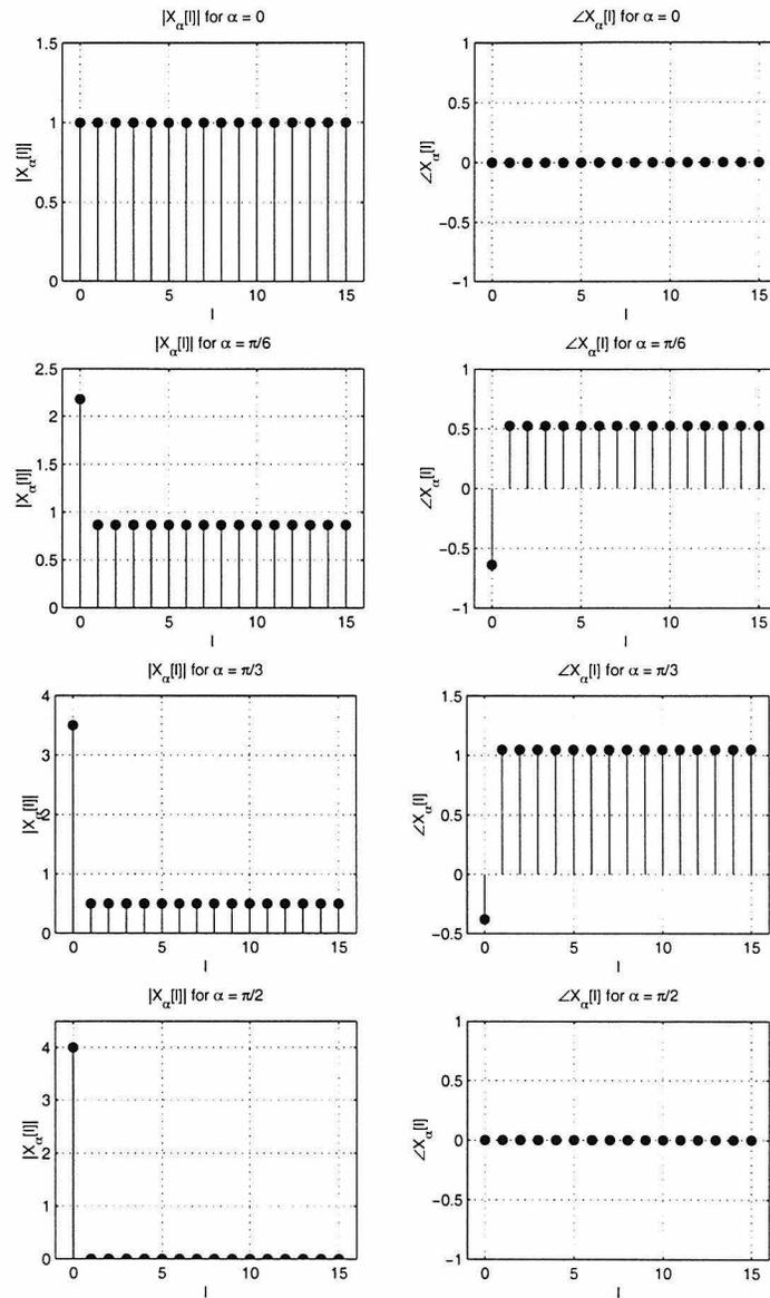
Figure 2.1: Magnitude and phase plots of  $X_\alpha[l]$  for various angles  $\alpha$ .
