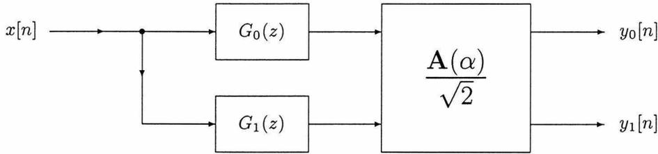
Figure 3.2: Implementation of two transfer functions by applying the FDFT to two allpass filters
