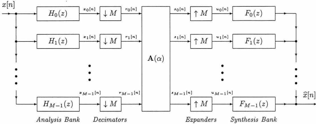
Figure 3.4:  $M$ -channel maximally decimated filter bank implemented with the FDFT
