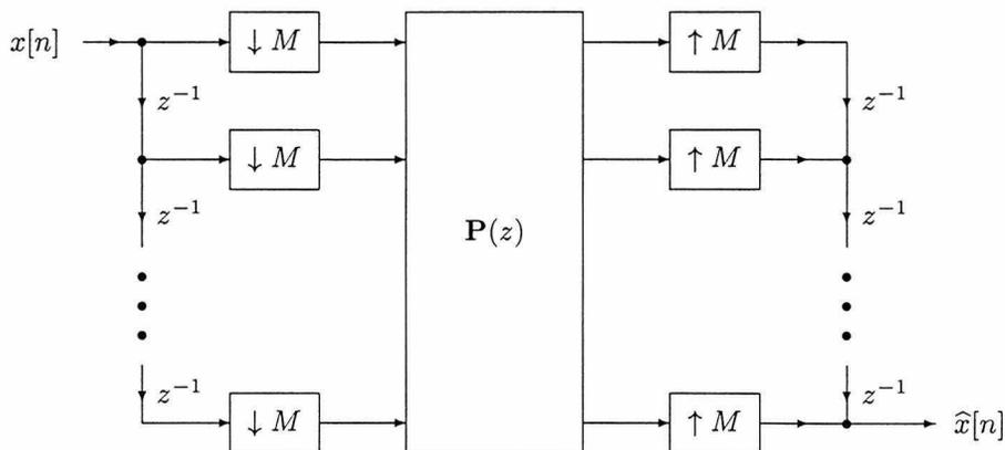
Figure 3.7: Canonical structure of the polyphase form of the  $M$ -channel maximally decimated filter bank
