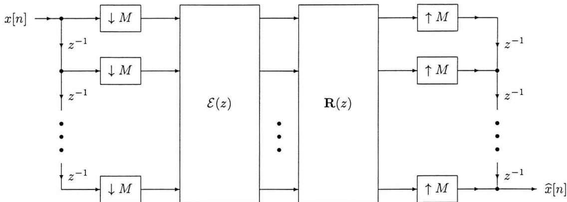
Figure 3.6: Simplification of the polyphase form of the  $M$ -channel maximally decimated filter bank using the noble identities
