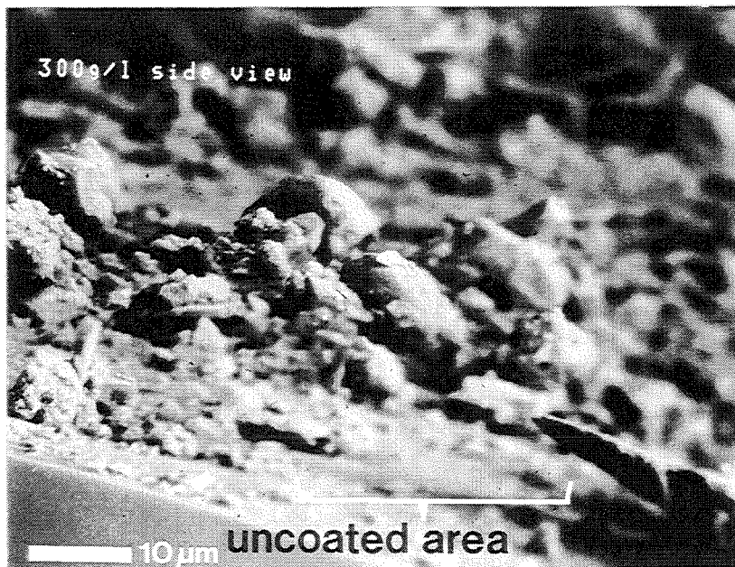
Fig. 3. SEM micrographs of Fe(III)-doped Q-sized TiO 2 on 1-mm diameter quartz optical fiber substrate: (c) 23 wt% coating, (d) oblique view.
