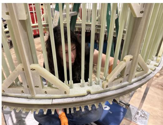
Figure 2.16: The author, sitting inside the the spin dressing magnet, while coiling the solder wire and inspecting the kapton tape to ensure it is covering the entire portion of the wire.
