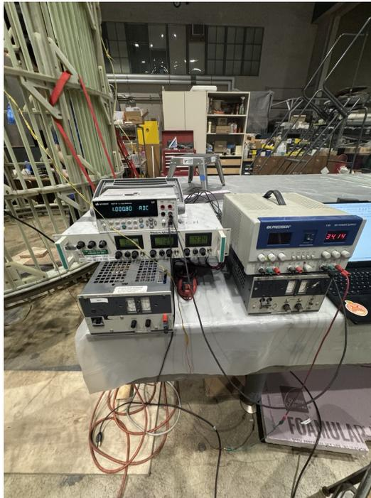
Figure 4.1: A photo of the power supply (top right), as well as the ammeter (top left) and magnetometer readout (middle left) used for taking the data of the magnetic field. The other two devices in the photo are non-functional power supplies.
