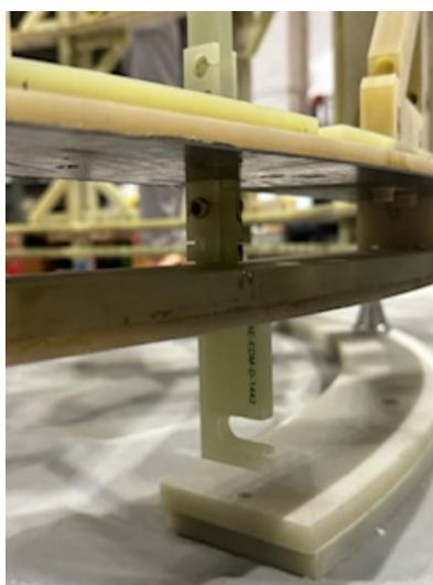
Figure 2.13: The bottom of the wire guide, showing the mechanism by which the wire guide is stabilized.
