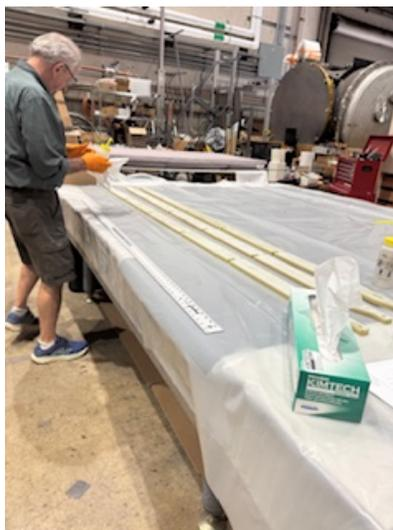
Figure 2.7: The story sticks being cleaned with isopropyl alcohol.
