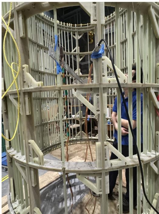
Figure 4.3: A photo of the experimental setup, showing the ruler across the x-axis of the spin dressing magnet, with the probe resting on the magnet.
