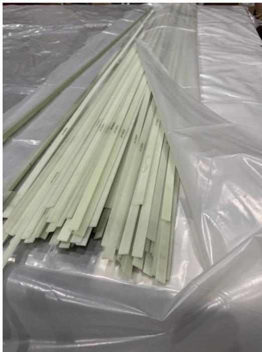
Figure 2.15: The wire guide caps, which are pieces of G10 that are slid into the wire guide slots, which cover the ridges in the wire guides that hold the wire and keep it in place.
