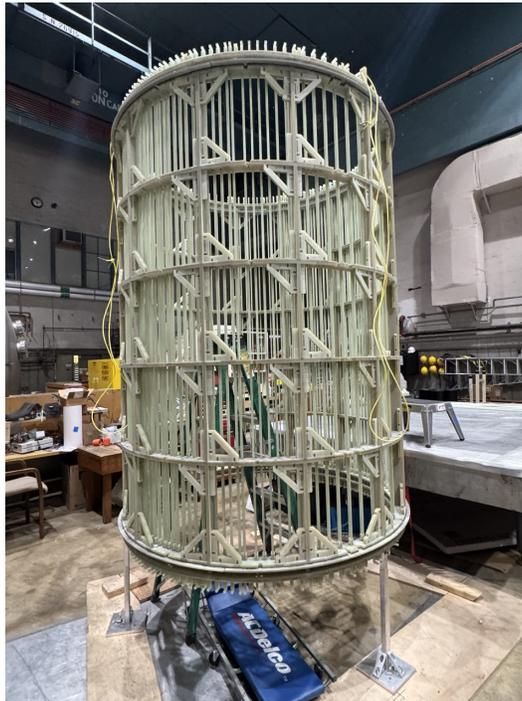
Figure 2.14: An image of the finished frame for the spin dressing magnet. The finished frame is all of the pieces of the frame without the wire wound or the wire guide caps.
