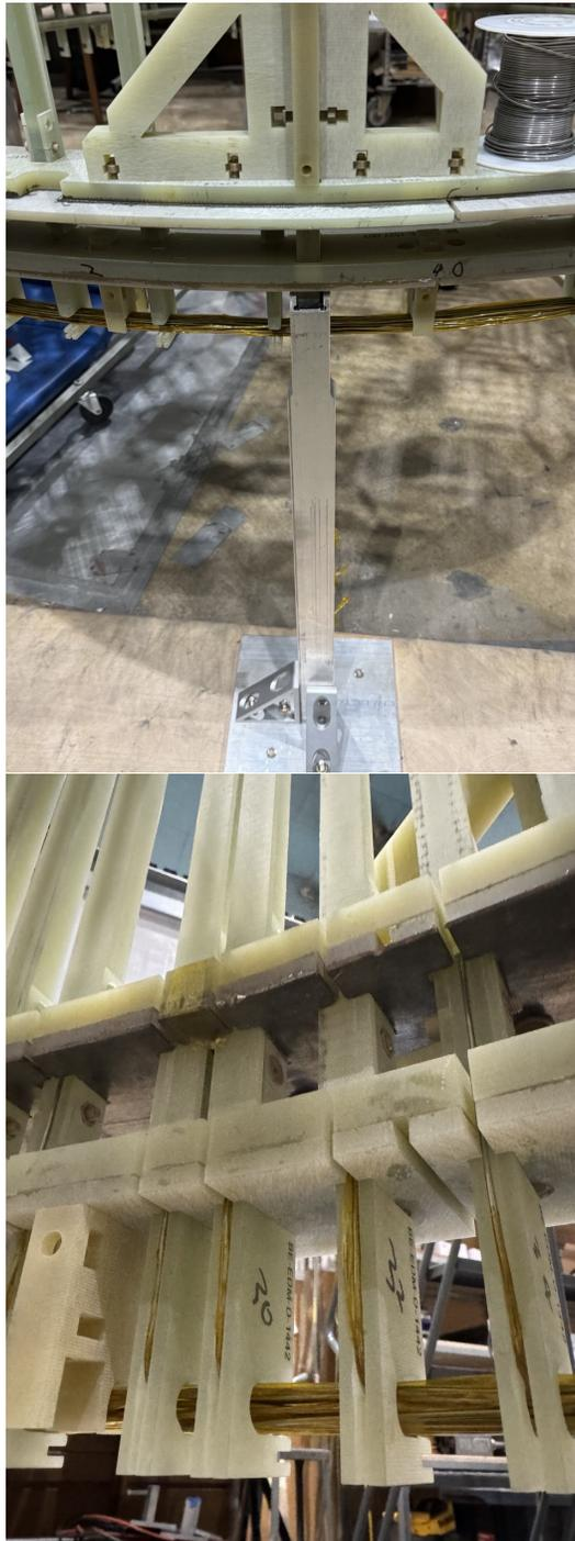
Figure 2.17: The wires along the saddle portion of the magnet. The golden-orange color is from the kapton tape coating the wire to prevent different sections of the wire from coming into contact with each other.
