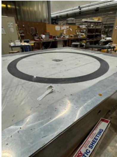
Figure 2.6: Lead was cut in the general shape of the bottom LEC and covered in epoxy glue. The LEC was later placed on top of the lead and the remainder was trimmed away. The LEC was then covered in plastic and vacuum sealed while the epoxy cured. Proper lead safety precautions were taken during this process, including using coveralls.
