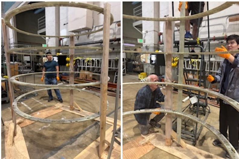
Figure 2.8: Images of the assembly of the spin dressing magnet frame. At this point in the assembly process, the rings are the only things assembled (left) and are resting on wooden scaffolding. In the right figure, a story stick is being inserted into the slot in the rings.
