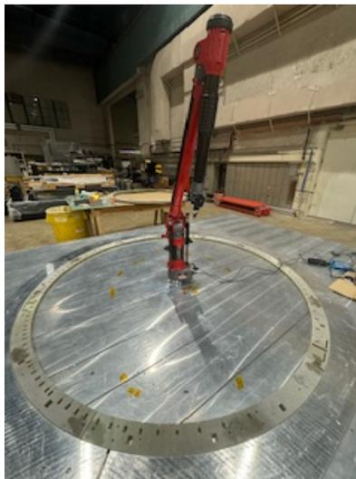
Figure 2.4: This image shows the ring in the brace on the table with the ROMER arm in the middle. To take the measurements, one person would be putting the measurement adapter into each slot, as well as ensuring that the correct slot is being measured. The other person must sit on the table and manually move the tip of the romer arm to the adapter in each slot and press the button to take the measurement.
