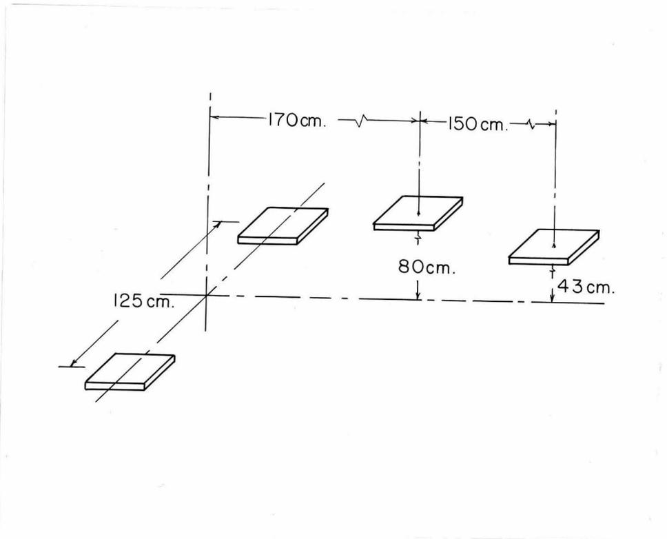
**Fig. 8.** Pictorial view showing position of trays for measuring wide showers. Arbitrary reference plane is 87 cm. above the floor of the plane, and the center tray is attached to the overhead.
