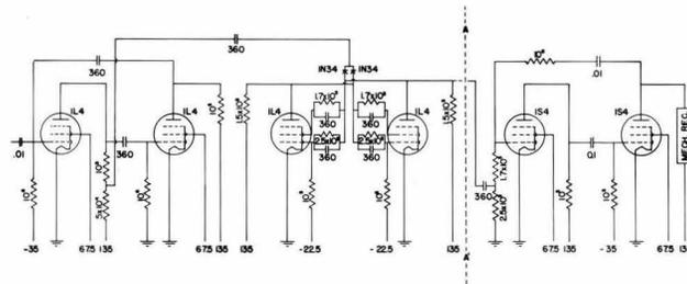
Fig. 7. Circuit diagram of scaling circuit used.
