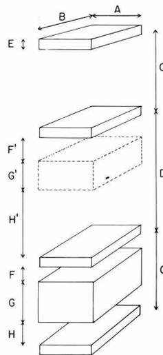
**Fig. 5.** Typical cosmic ray telescope used in airplane flights.
