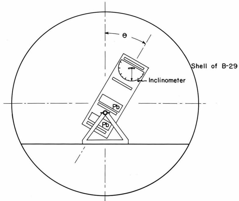
**Fig. 6.** Pictorial sketch showing method of mounting cosmic ray telescopes in airplane.
