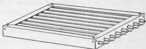
FIG. 2. Eight counters were mounted rigidly in a framework to form a sensitive area of 600 cm<sup>2</sup>. Three of these trays were used to count triple coincidences. The weight of each tray was 850 g.
