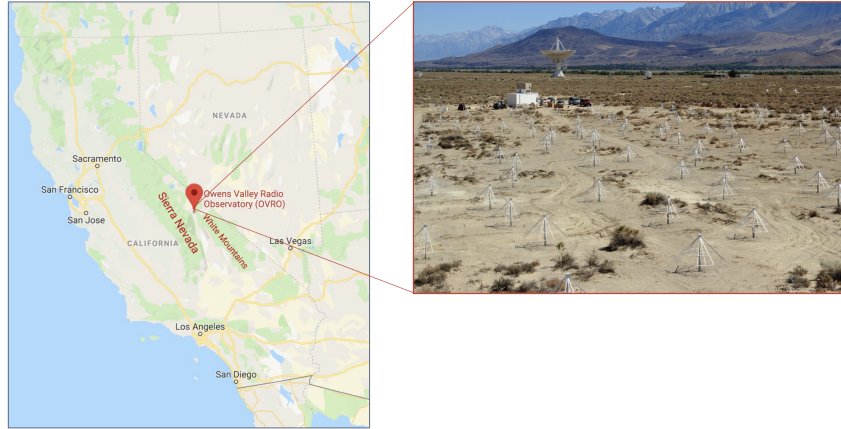
Figure 1.6: Location of the Owens Valley Radio Observatory and a photo of the cross-dipole antennas of the OVRO-LWA. For scale, the length of each dipole arm is about 1.5 meters. The white shipping container in the back hosts the electronics and computing cluster that processes the data.
