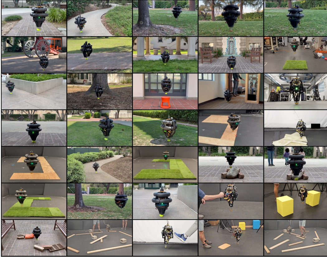
Figure 8.1: A snapshot of the experiments conducted with ARCHER, including path planning, disturbance rejection, and hopping over rough terrain.
