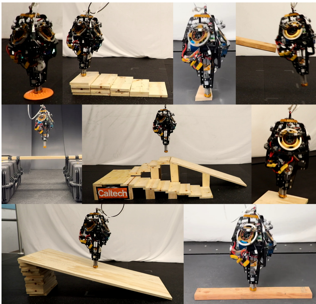
Figure 5.21: A snapshot of the experiments conducted with ARCHER, including set point tracking, disturbance rejection, and hopping over rough terrain.
