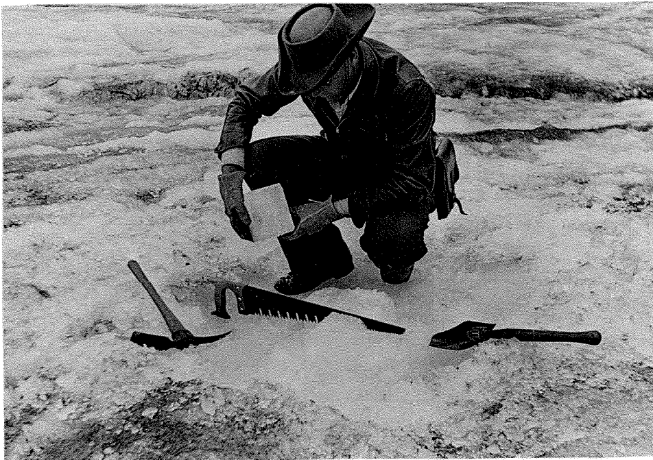
Fig. 3.- Method of cutting out ice blocks previous to making thin-sections. Photograph by B. H. Bieler.
