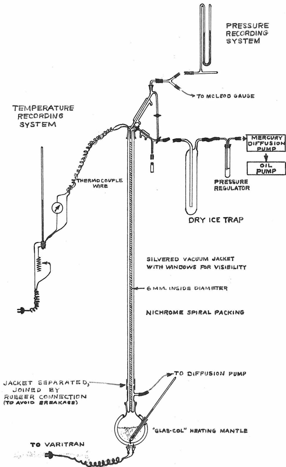
Fig. 33. High Precision Fractionation Apparatus.
