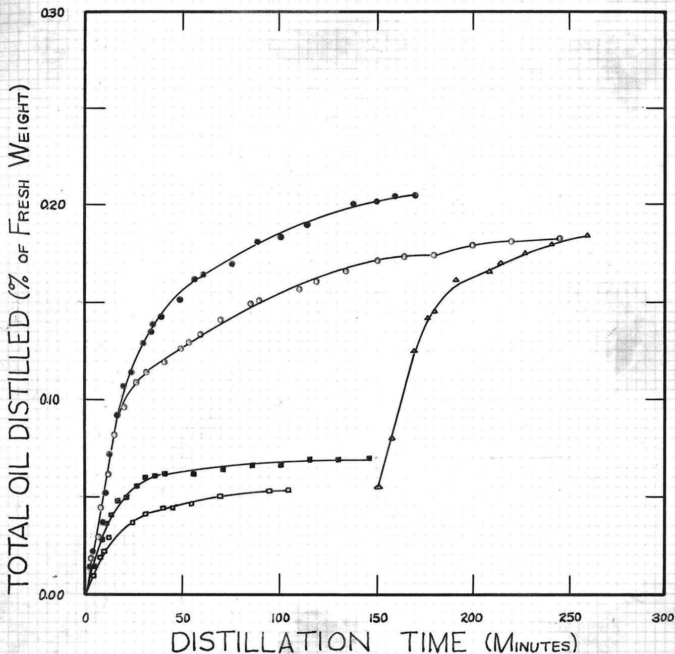
Fig. (1). Sharp Morphological Fractionation; Steam Distillation of Four Year Guayule Stems.
