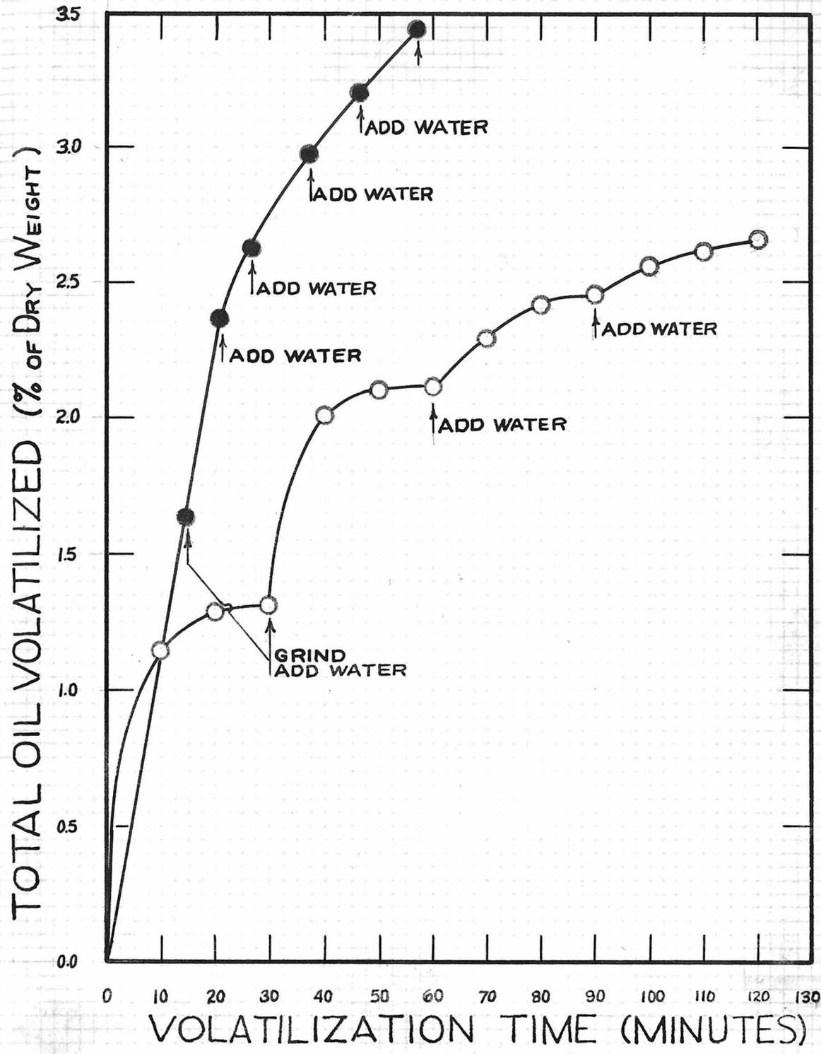
Fig. 17. Reduction of the Total Time Required for Exhaustive Volatilization.
