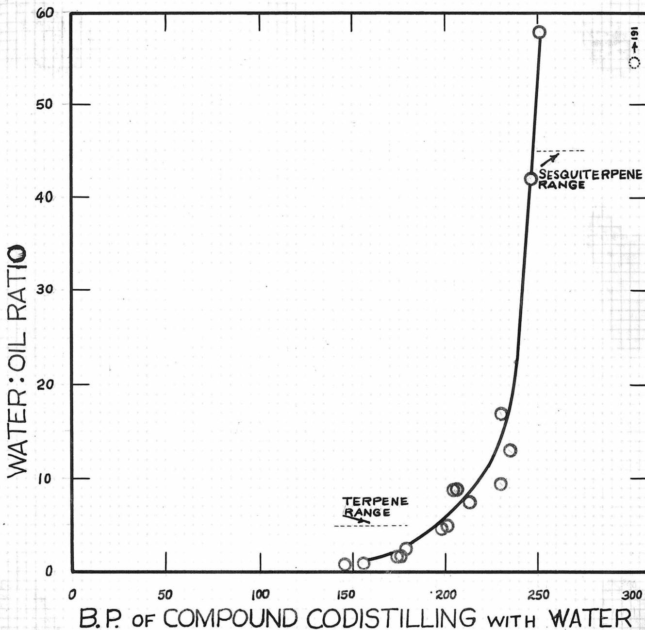
Fig.(9). The Compositions (Water:Oil Ratios) of Various Codistilling Systems of Water and an Immiscible Organic Compound as a Function of the Boiling Points of the Organic Compound.
