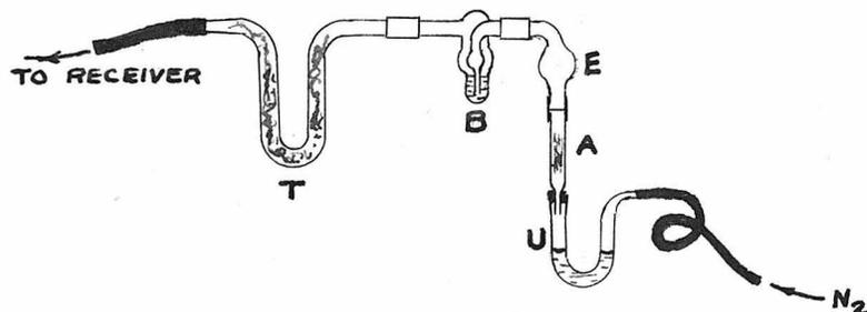
Fig. 18. Apparatus for Aeration of Carbon Dioxide from the Absorption Tube.
