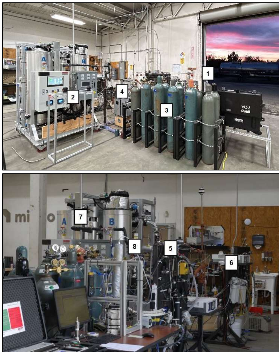
Figures 2.5 and 2.6 display the complete Centennial system from two different angles. The cooling tower is around the open door (1) in Figure 5, and thus not displayed. In Figure 5, the tower control panels (2) are displayed on the reactor front, as well as compressed gases on the right (3), which are used to generate different flue gas conditions. In between the towers and cylinders sits a steam generator (4) used primarily to humidify the flue gas. Occasional trials were conducted where steam was also utilized for CO 2 regeneration. In Figure 6 the gas mixing (5) and gas analysis (6) panels are visible. An in-line heater (7) is available near the tower control panels and provides extra temperature control for injected flue gas. One of the water-cooled heat exchangers (8) also illustrated in Figure 2.3, is visible to the left of the gas mixing panel.
