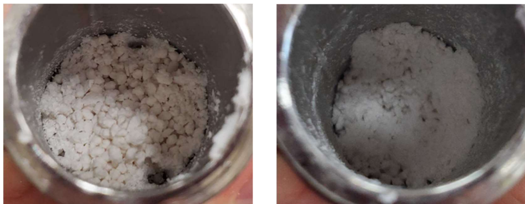
Figure 3.6 displays examples of unstable material after exposure to the humidification cell. The left shows what particle clumping looks like. The right shows dissolved/deteriorated sorbent. Both samples are from the A series and have an appearance typical of sorbents which do not contain dessicant.
