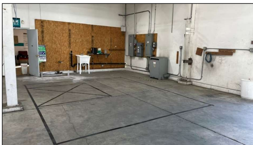
Figure 2.4 shows the Centennial site prior to construction. Black tape was used to outline the approximate total system size. The black “X” indicates the approximate site the skid-mounted towers were placed. Component placement was optimized according to the location of the water supply (the white sink), site drainage (the black tube by the sink), and power supply (transformer and electrical control panels, grey).
