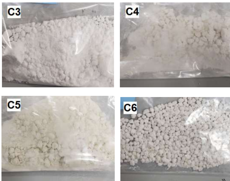
Figure 3.9 displays samples C3-C6 after 33 cycles on the auto cycler. C6, which contains 13X exited the cycler with minimal decomposition, clumping, or dust formation.
