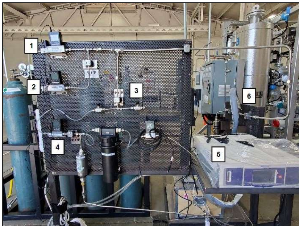
Figure 2.7 shows the original perforated panel design. Two mass flow controllers set the flow of CO 2 (1) and N 2 (2) coming from pressurized cylinders. Around 2 lpm of the mixed “flue” gas is sent to a CO 2 analyser (5) via another mass flow controller (4) to monitor composition changes in real time. Again, this is not as necessary when flue gas is generated by controlled gas mixes, but later compressed ambient air was used instead of N 2 to increase flow rates. A pressure relief valve (3) can be used in case of an emergency shutdown. Once the gas is mixed and analysed it is sent to a junction (6) that introduces water vapor from the steam generator.
