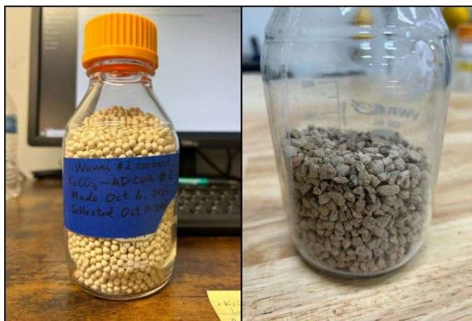
Figure 2.12 displays the Mitico-prepared ADCOA spherical zeolite (left) as well as the PureAir-prepared rock-type zeolite (right).
