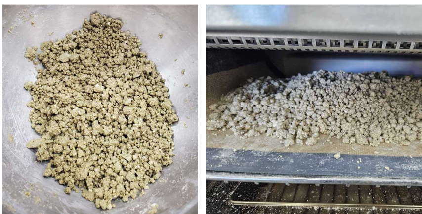
Figure 3.3 shows an example of particles formed from this process. The left panel shows wet particles still in the bowl of the stand mixer. On the right are the particles spread thin on a baking sheet after 2 hours in the convection oven. Wet granulation is a robust process; while the particles formed may not have regular size and shape distributions, coagulation through mixing and compaction works for most formulations (and worked for all formulations presented here).
