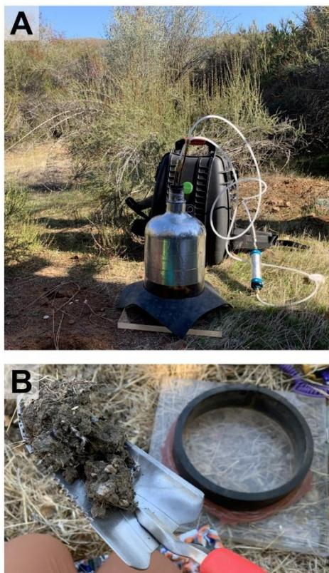
Figure 6.1: Components of kinetics measurement system. A: Measurement system during a kinetics measurement. Chamber is fitted into the chamber base, with a neoprene skirt covering the juncture between chamber and chamber base. Chamber is connected to the field-portable CRDS analyzer inlet and outlet via two lengths of tubing and an inline water trap. B: Detail of chamber base, a Neoprene collar fixed to an acrylic sheet with butyl rubber adhesive.
