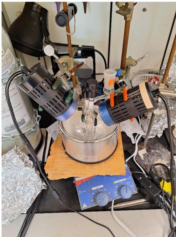
**Figure D1:** Typical setup for catalytic experiments. Lights are turned off for clarity.
