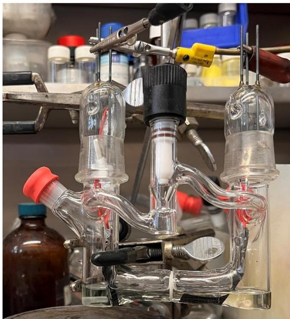
**Figure E1:** Two-compartment cell used for CPE experiments.
