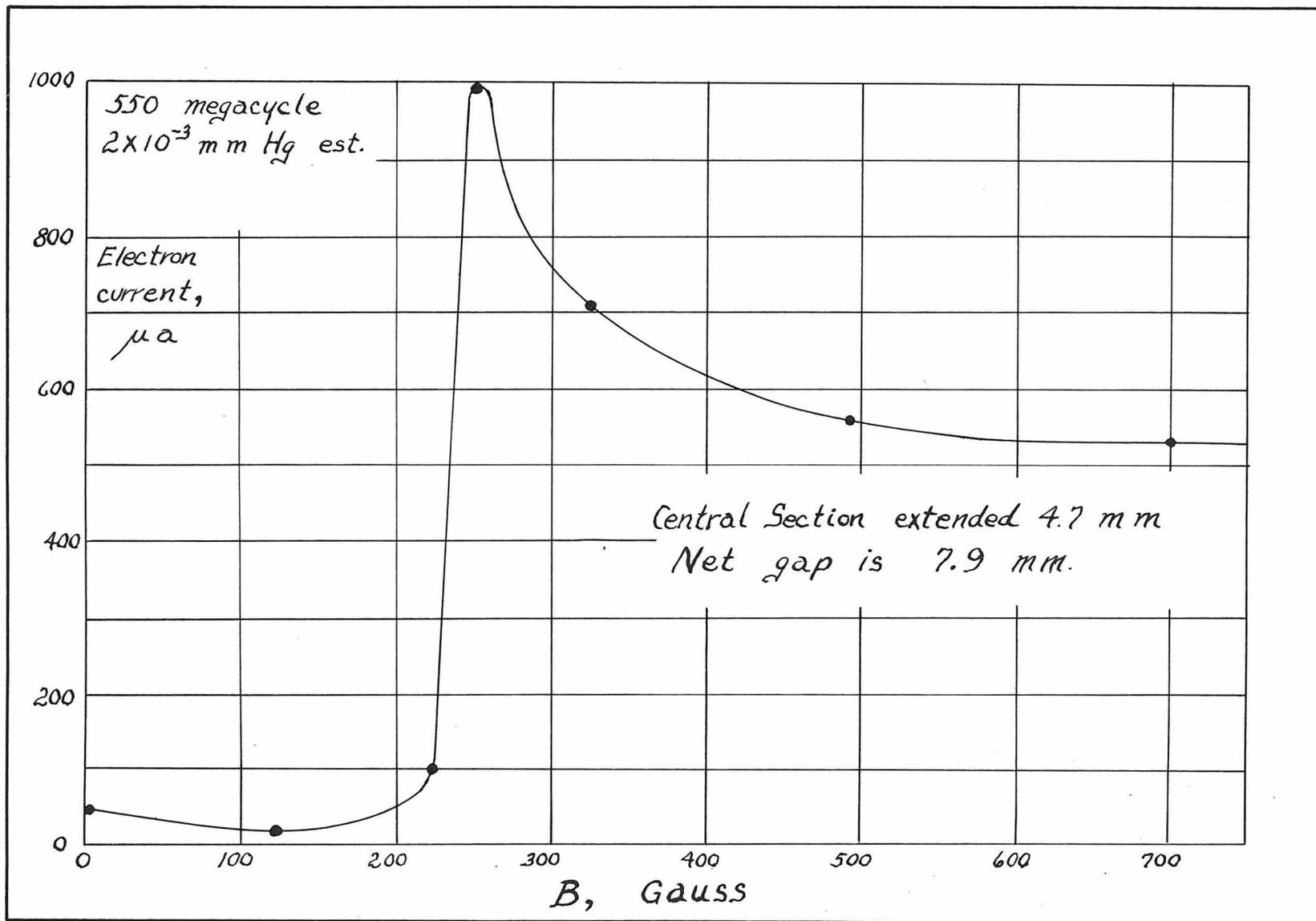
behavior seen here; the electron density will increase sharply at the point where the average electron energy is high enough to be effective in producing secondaries, but the imposition of higher than optimum magnetic fields will depress the yield of electrons because the space charge eventually becomes so high that the low energy secondaries cannot get across the gap to contribute to the process.
