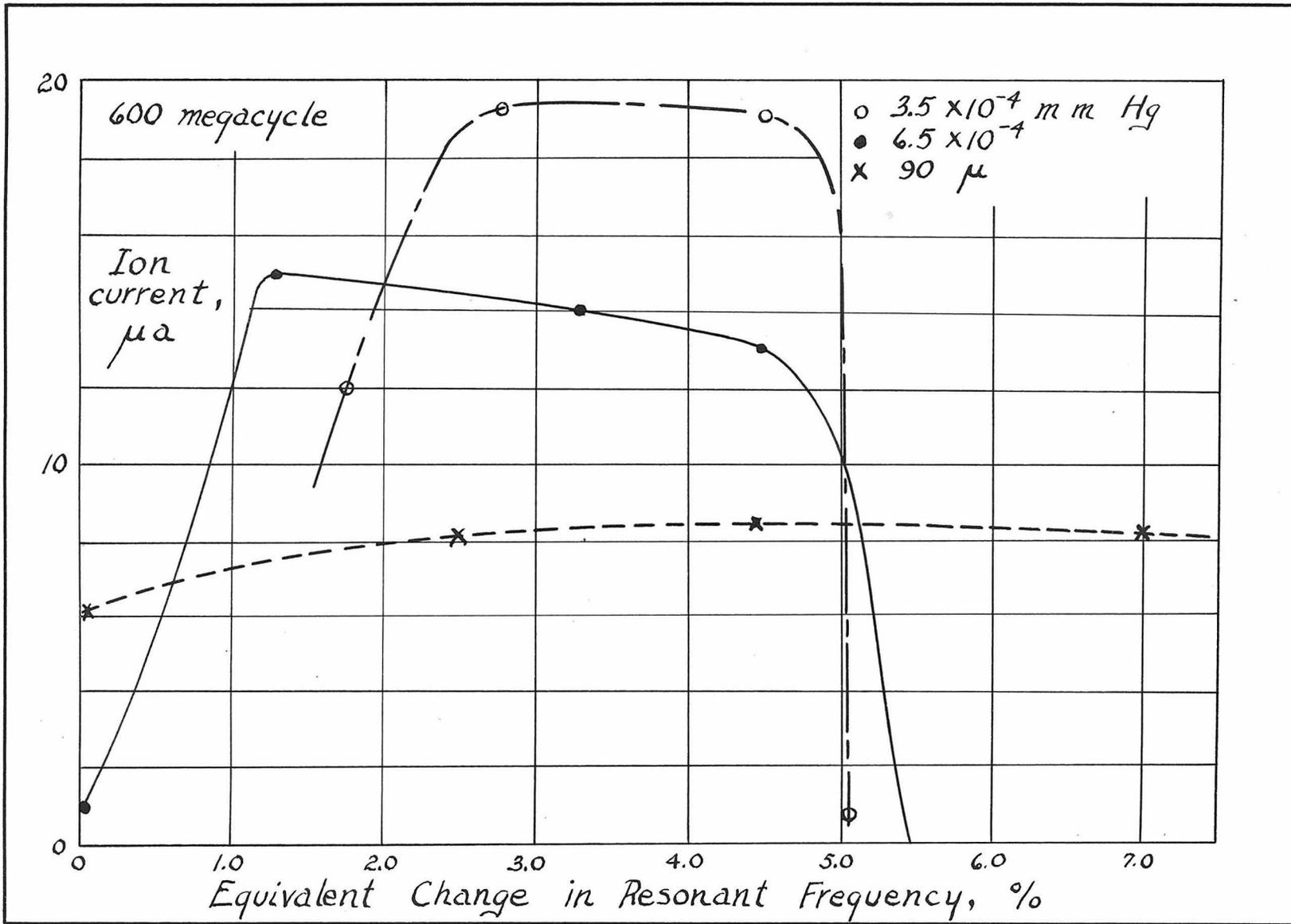
characteristics to tuning plug position at high pressures would seem to be very clear. This is easily explained on the basis of a broadening of the cavity resonance curve by a dissipative load, by which the ionization processes in the discharge may of course be represented.
