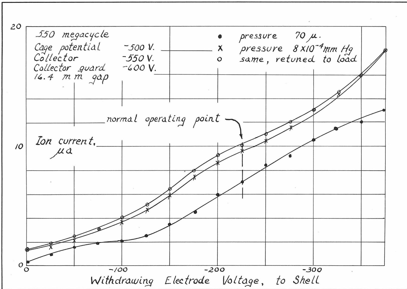
charge effect is involved; the fact that the ion current rises monotonically while the withdrawing electrode potential is taken all the way from the source cavity potential to the Faraday cage potential indicates against the supposition that the rise can be due entirely to a focussing effect.
