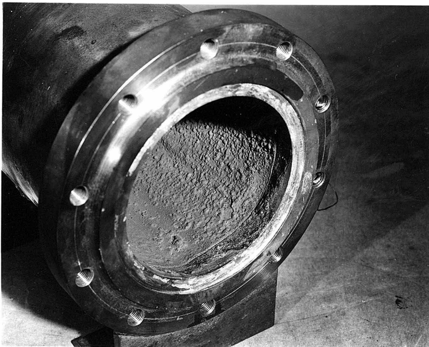
Figure 30--Photograph from nozzle end showing zirconia liner after tests B-82-N & B-83-N. Note that melted zirconia has been scraped off the lip of the casing. Note also that casing lip has been melted during these tests. (This lip was removed in later redesign of chamber casing.)
