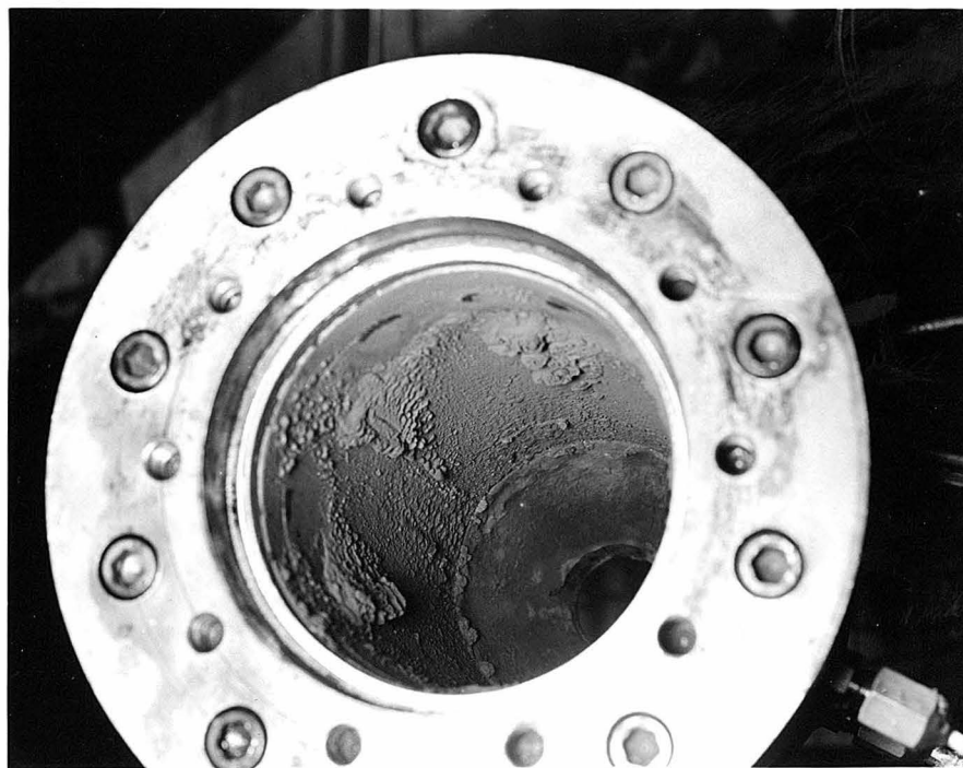
Figure 41--Photograph showing deposits on silicon carbide liner after test B-94-N. Also see figure 40.
