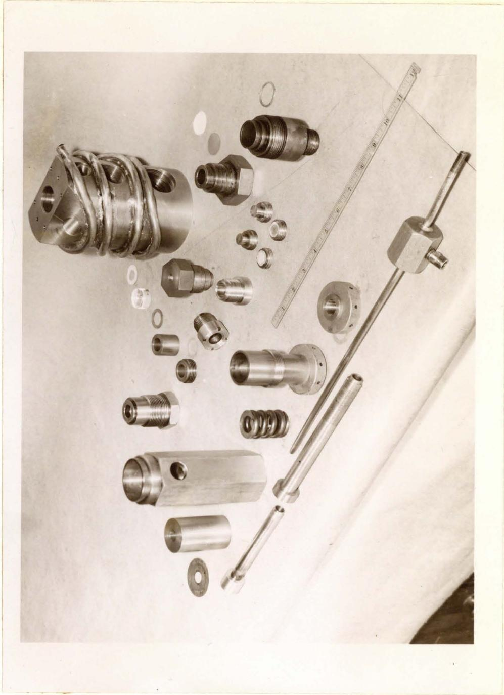
Figure 17. View of Continuous Reaction Chamber and Control Valve.
