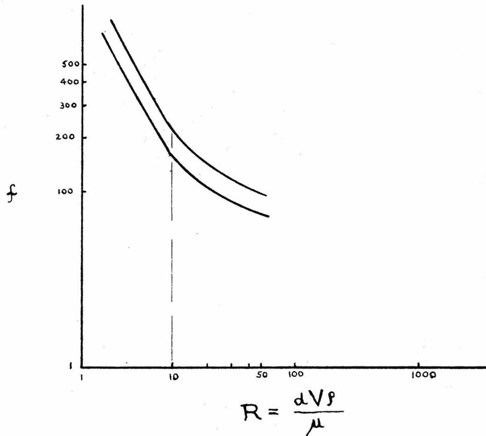
The break in the straight-line portion of the curve occurs in the vicinity of  $R = 10$ . This indicates that if  $R$  is greater than 10, the flow is turbulent.
