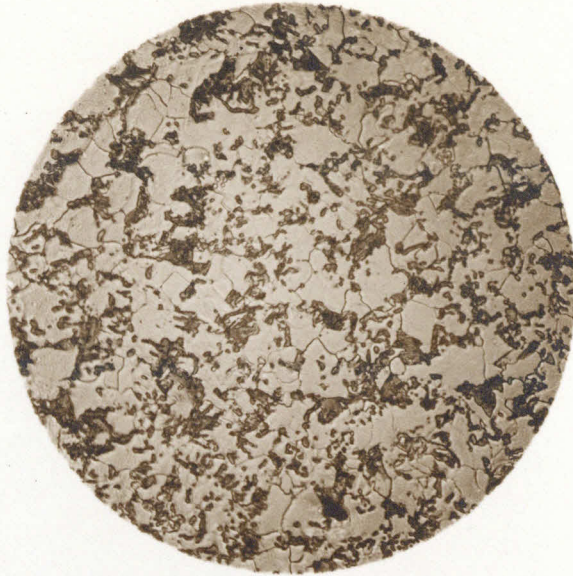
Fig. 28a. Specimen Steel SAE X 4130 at 500 X, Nital Etch.
