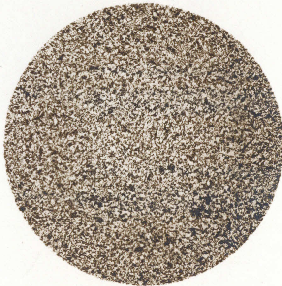
Fig. 28b. Specimen Steel SAE X 4130 at 100 X, Nital Etch.
