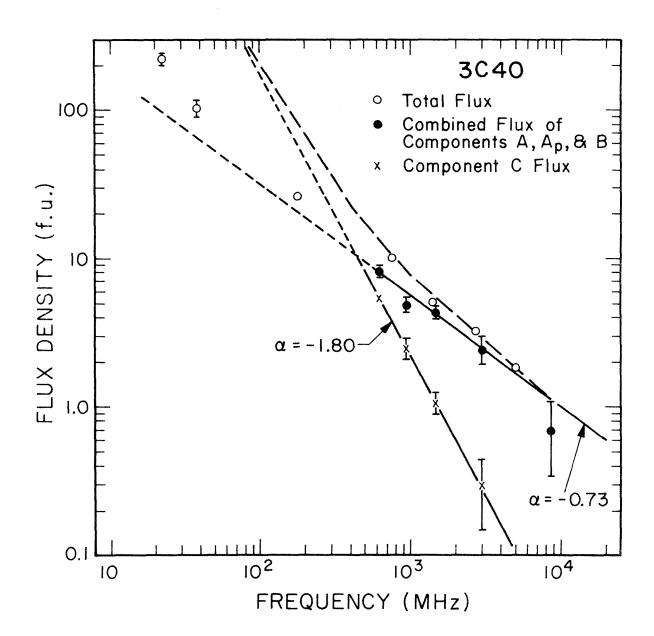
References for the component flux densities are given above. The total flux densities are from Roger et al. (1969) at 22.25 MHz and the rest from Kellermann et al. (1969). Since the sum of the power law spectra extrapolated to low frequencies does not fit the observed total flux densities one or both of the component spectra must flatten below 600 MHz.
