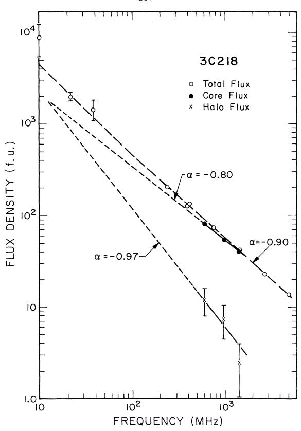
5000 MHz. Two power law spectra are used to fit the core flux densities and a single power law spectrum for the halo. Although the spectrum of the halo is very poorly determined due to the large flux density errors, the combined spectrum shown in Figure 14 agrees rather well with the observed total flux densities. Since there are no low frequency measurements of the component fluxes, their spectra could be more complicated than shown at frequencies below 600 MHz.
