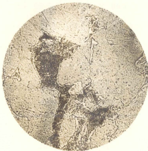
Figure 9. Silver-Copper Steel Magnification 500x As Cast
