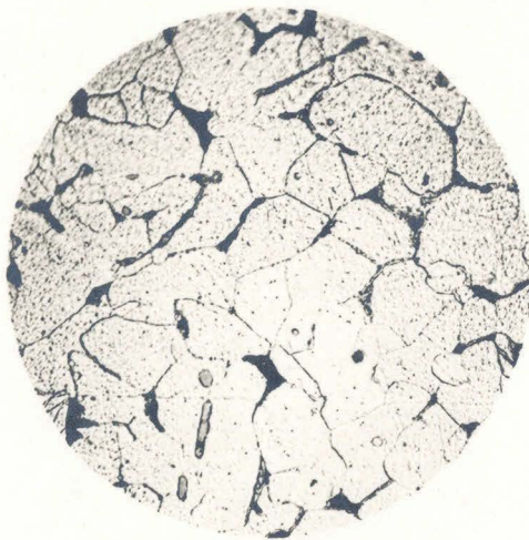
Figure 3. Mild Steel Containing 0.015 per cent Silver Magnification 500x As Cast
