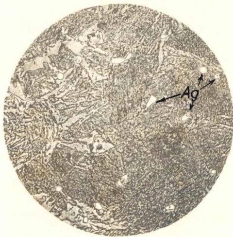
Figure 8. Silver-Copper Steel Magnification 500x As Cast
