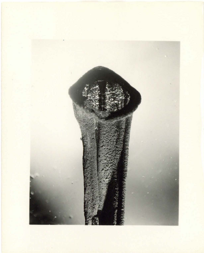
fig. 5. Silver skeleton from ashing W3B impregnated carbon. 6.2 magnification.
