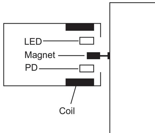
The arm cavity OSEMs (Fig. 4.8) are similar, only they have a single photodiode instead of a split photodiode. For both types, the effect of the local damping system is to reduce the pendulum
