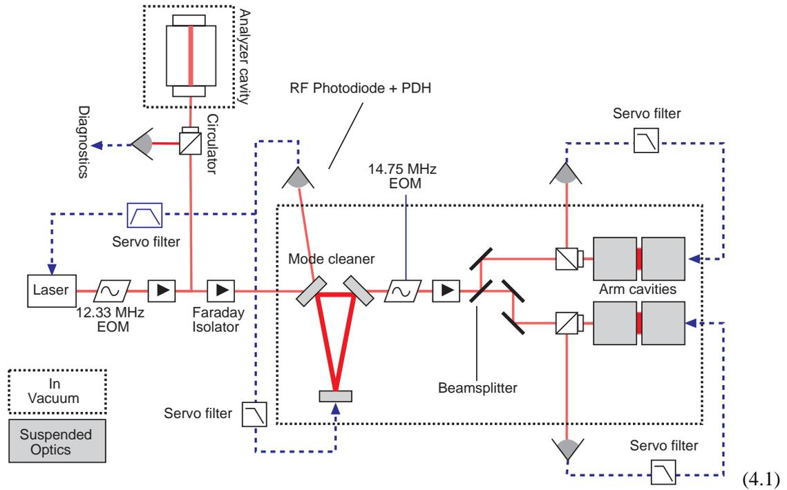
mirrors have local damping servos to reduce the pendulum  $Q$ , but the servos roll off strongly above 20 Hz so that the mirrors are essentially free masses above 300 Hz.
