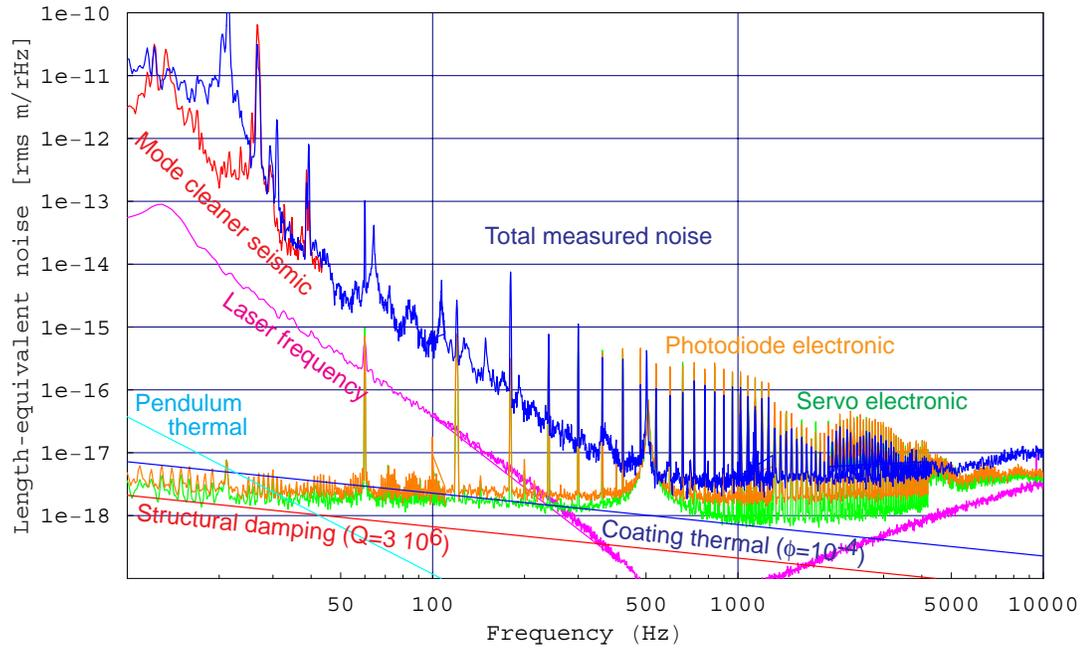
Figure 4.11: South arm cavity sensitivity. [16]
