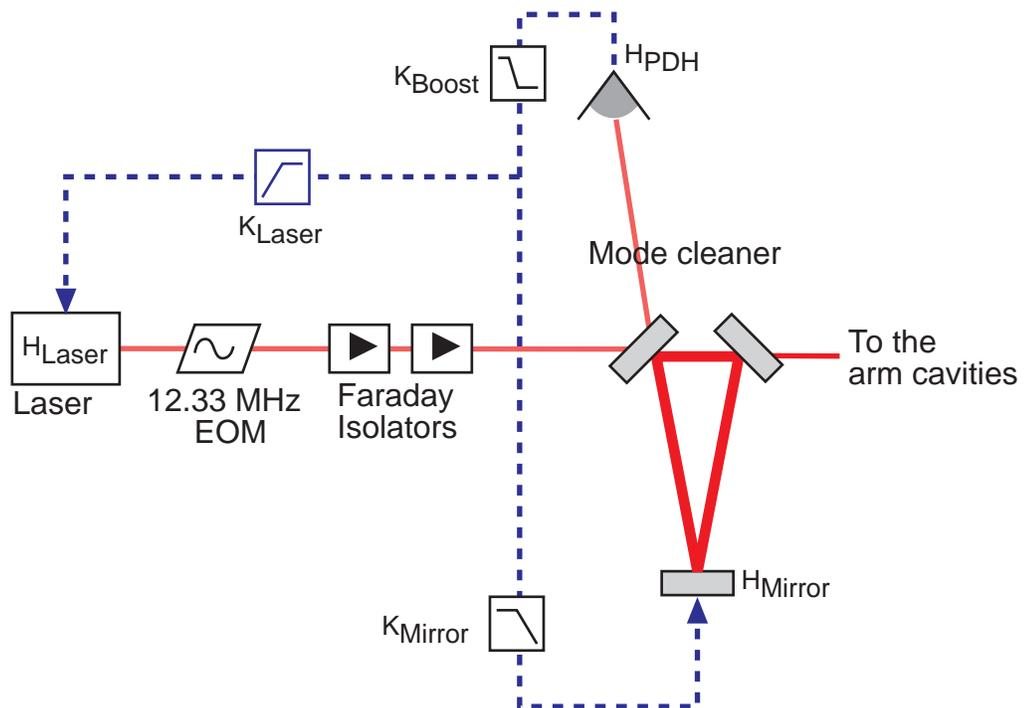
The laser PZT bandwidth is 120 kHz [75], which allows frequency noise suppression up to 90 kHz (see §4.3). If the servo gain is raised so that the unity gain frequency is higher than 90 kHz, servo oscillations occur. Schematics of the servo electronics are documented in LIGO technical notes T000077 and T010023 [18, 17].
