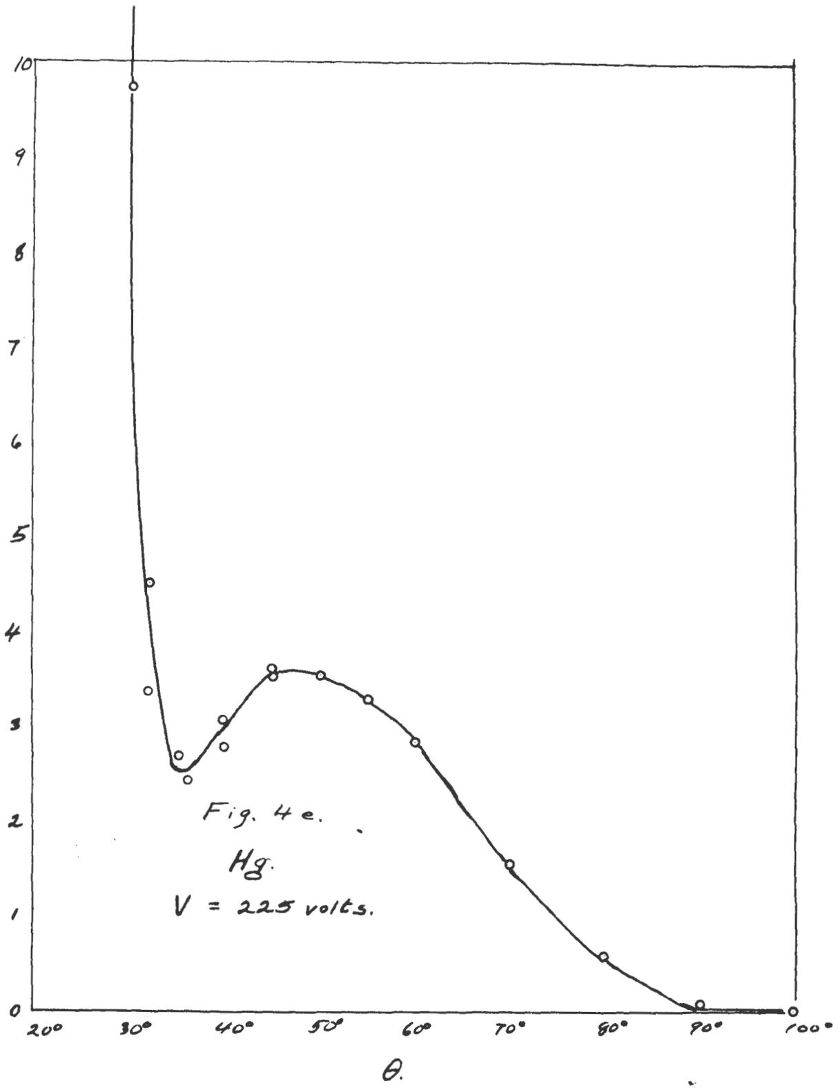
The angular setting of the collector could be done with an accuracy of approximately a degree. The pointer setting, of course, would be accurate, and the backlash was small. The possible error lay in the centering of the  $0^\circ - 180^\circ$  line of the scale with the direction of the main beam. This was done visually, and checked by scattering measurements at positive and negative angles.
