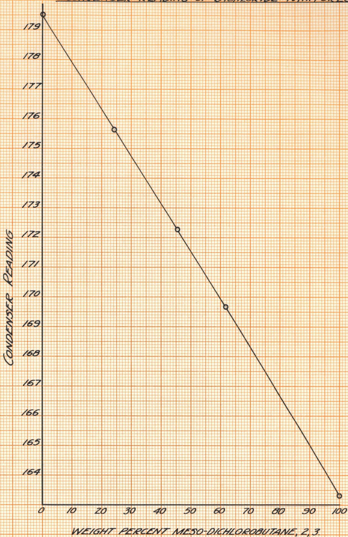
FIGURE 1. CONDENSER READING OF DICHLORIDE MIXTURES
