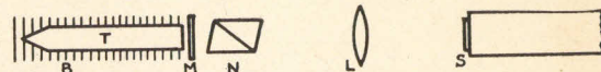
FIG. 1. Experimental arrangement for polarization measurements. M , half-wave mica plate; N , Nicol prism; S , step weakener on slit of spectrograph; T , Raman tube; L , condensing lens; B , parallel black screens.
