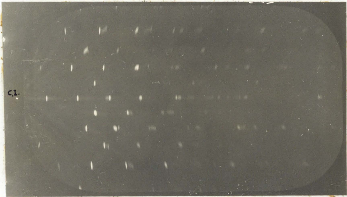
Oscillation Photograph Reflecting \text{CuK}\alpha from (110)_{rh}
