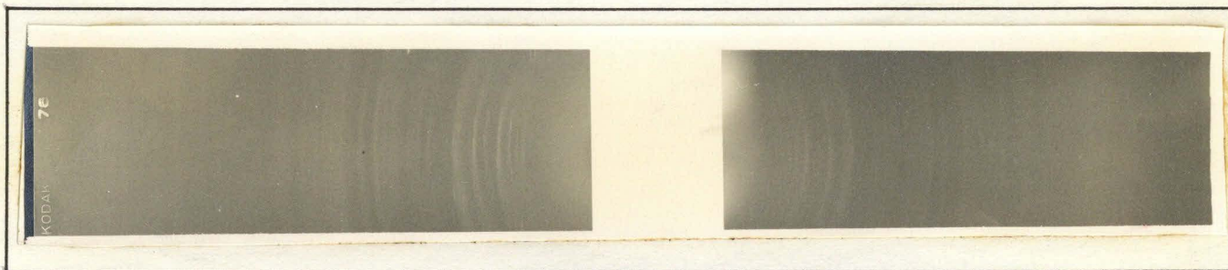
FIGURE 6e -- Powder photograph of \alpha - monoclinic selenium, obtained from powder resulting from a single crystal.
