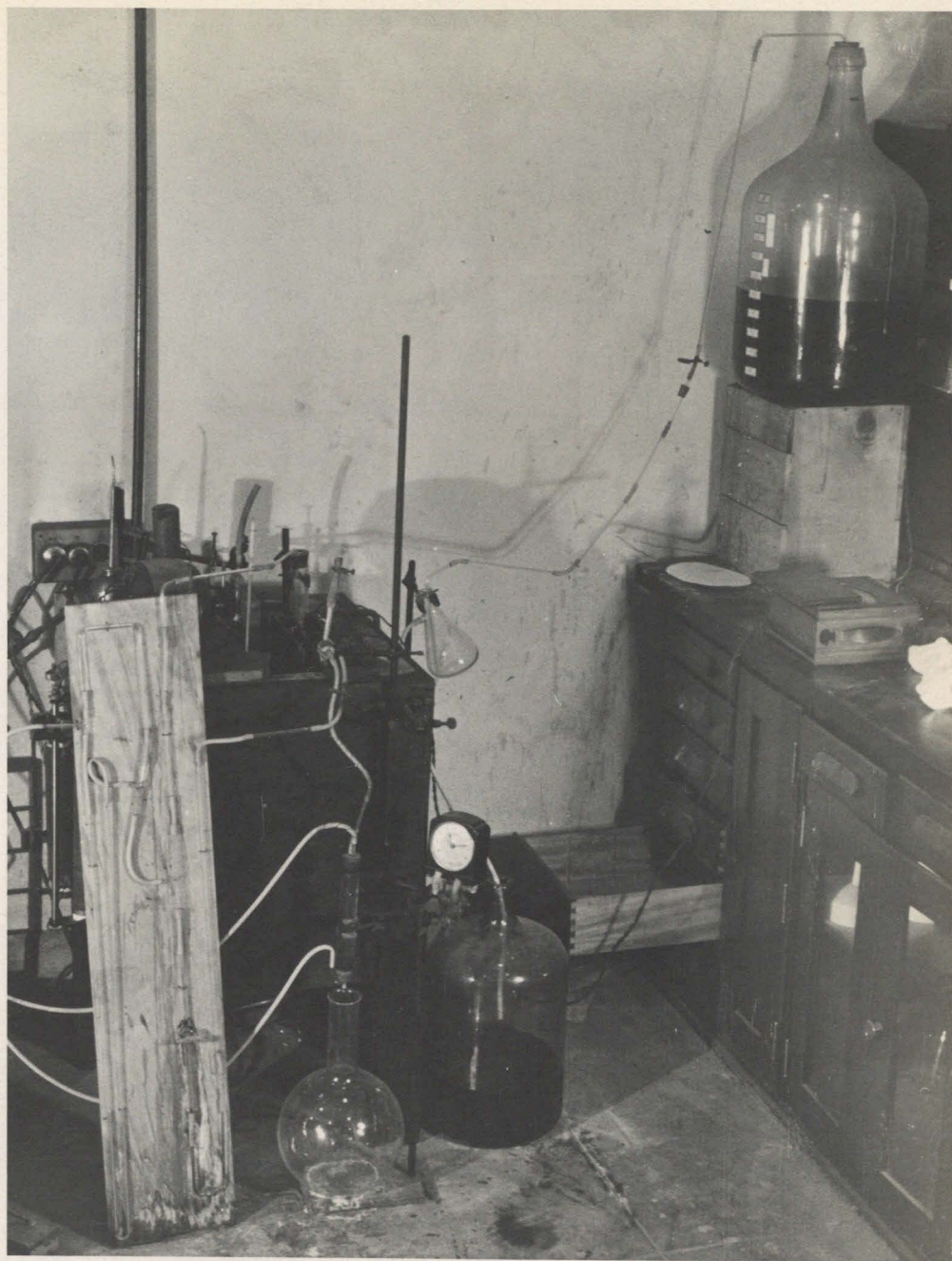
Fig. 3 Assembled Apparatus, Showing Feed and Circulation Systems
