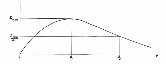
All the lightning surges induced on lines have a very close shape to the double exponential wave :
