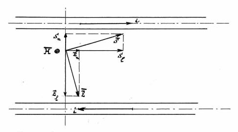
We shall be interested in the case of a double wire line. We suppose that the conductors are so remote from each other that the current flowing in each wire has no effect whatever upon the distribution of the current in the other. In other words, the skin effect in each conductor will be the same as if it were isolated; this approximation is excellent.
