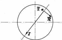
The Poynting vector, inside of the wire, is radial and directed toward the center, as can be seen at once.
