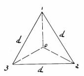
It is impossible to speak of the self inductance of a three phase line in general, since there are three wires carrying three different currents.
