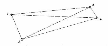
Let the two loops be (1,2) and (3,4), having unit length. The mutual inductance is the flux in loop (3,4) due to the current of unit value in 1 and 2.
