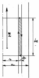
Another closed path is shown here. The supposed direction for  $\overline{E}$  implies a magnetic field into the paper. In order that the positive normal to the circuit be in the same direction as  $\overline{H}$ , we have to consider the direction of circulation as shown by
