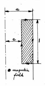
We consider the finite circuit between the radii r and a. By Maxwell's first law:
