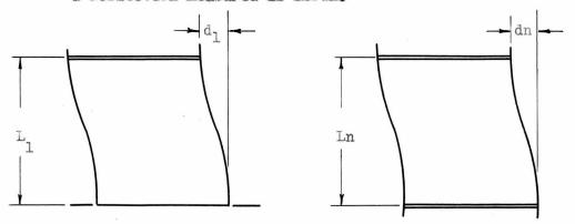
The same force was then applied to one of the upper floors, the floor immediately below being held stationary, and the deflection measured as shown. then
