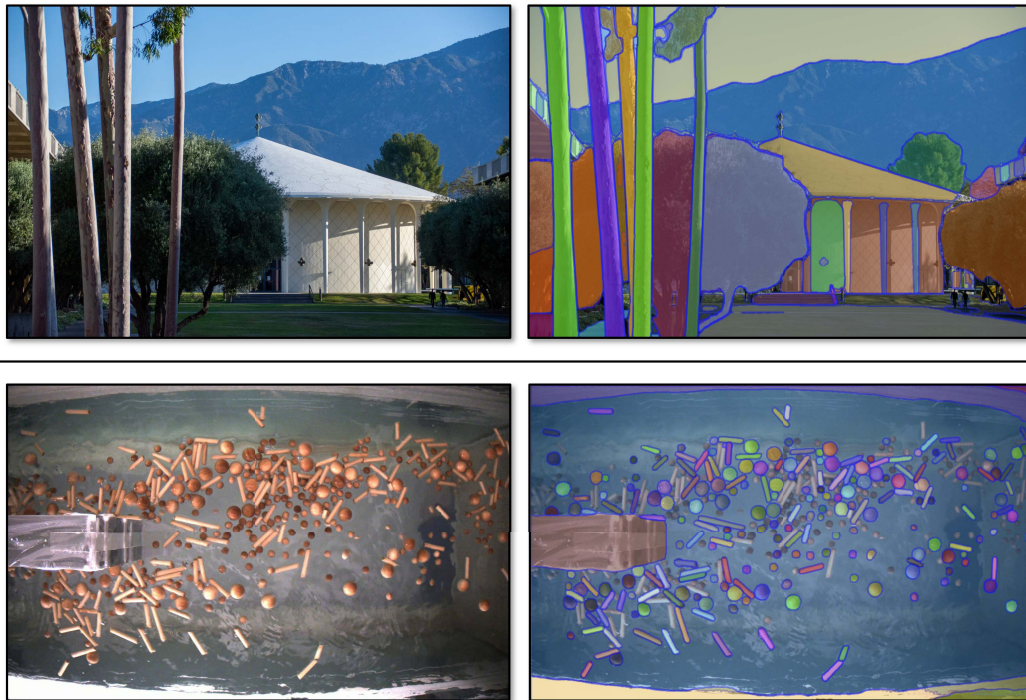
Figure B.3: Using Segment Anything Model (SAM, [155]) to identify and mask semantic objects within an image. Top: An image of Beckman Auditorium at Caltech. Bottom: A sample image from the experimental data presented in Chapter 5. Left: Original images. Right: SAM used to identify all semantic masks in an image based on the online demo implementation provided at https://segment-anything.com/
