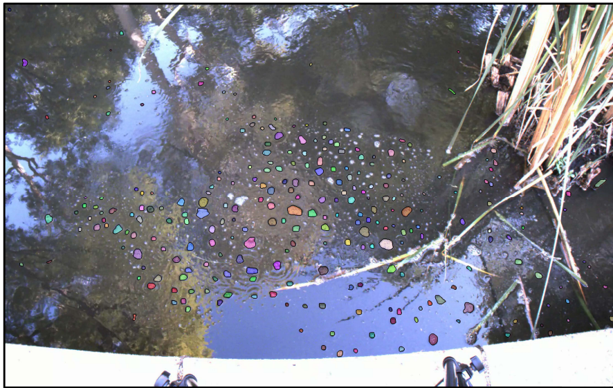
(a) A sample image from the data set with all detected surface tracer segmentations provided with randomly generated colors.
