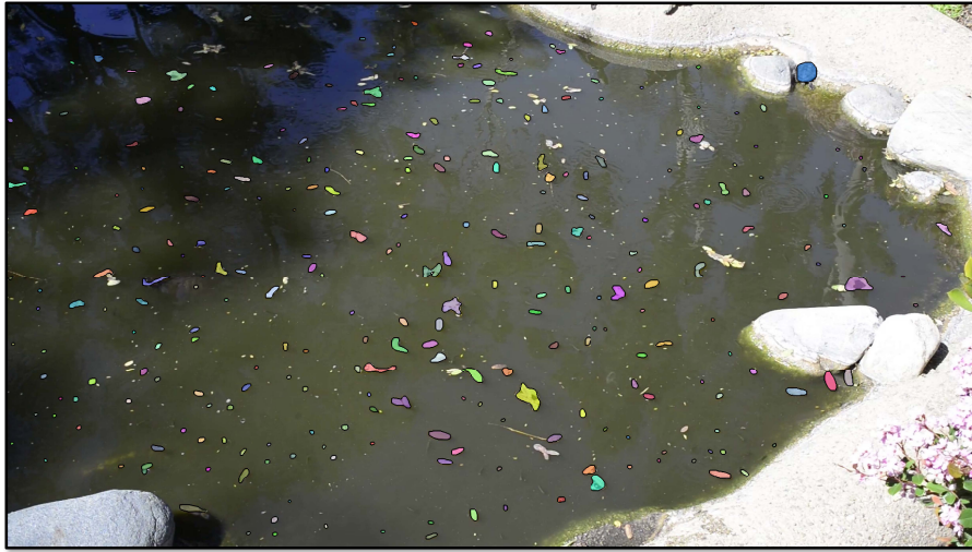
(a) A sample image from the data set with all detected surface tracer segmentations provided with randomly generated colors.
