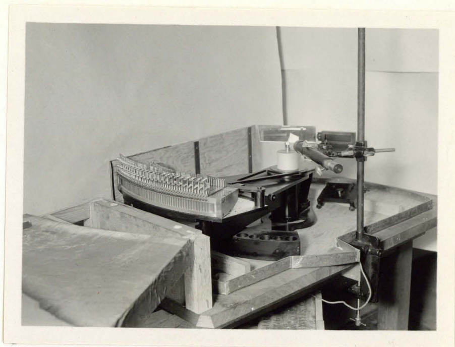
Fig. 12a. Showing small mirrors mounted on crystal holders, larger central, rotating mirror, and telescope. The scale was located behind behind the camera.
