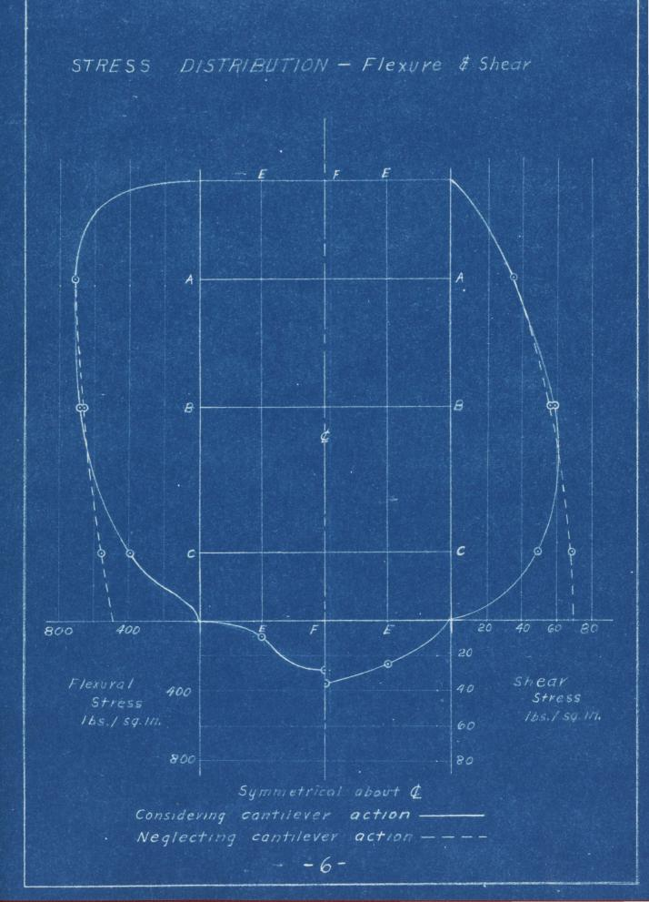
DIVISION of LOAD This diagram shows the division of load between the horizontal beam and vertical cantilever systems.
