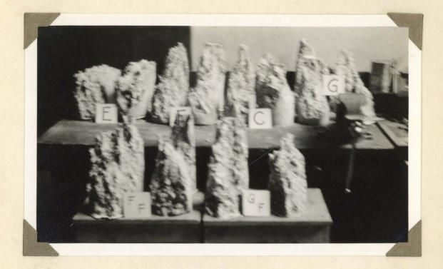
TESTED SPECIMENS PREPARED ACCORDING TO FULLER'S CURVES
