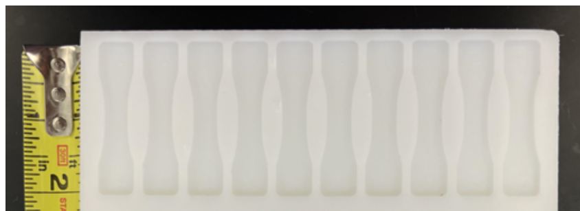
Figure 2.1: HDPE curved dogbone molds used for LCE synthesis.
